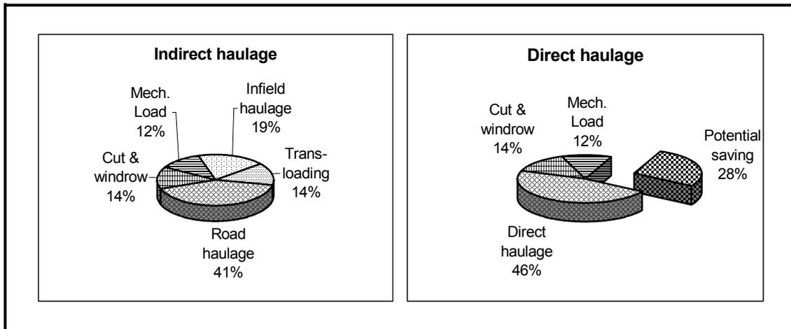
Figure 7. Indirect versus direct harvesting, loading and transport costs (Meyer, 2005)
