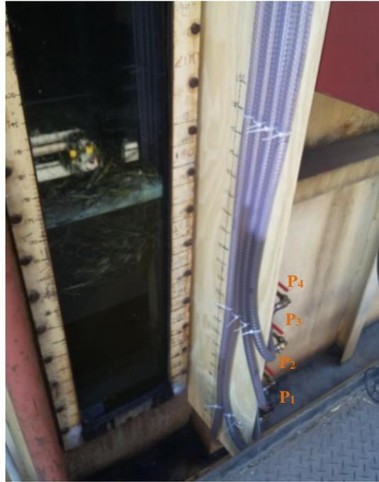
**Figure 1. Installation of the manometers in the wall of the diffuser and plastic tubes used as manometers.**
