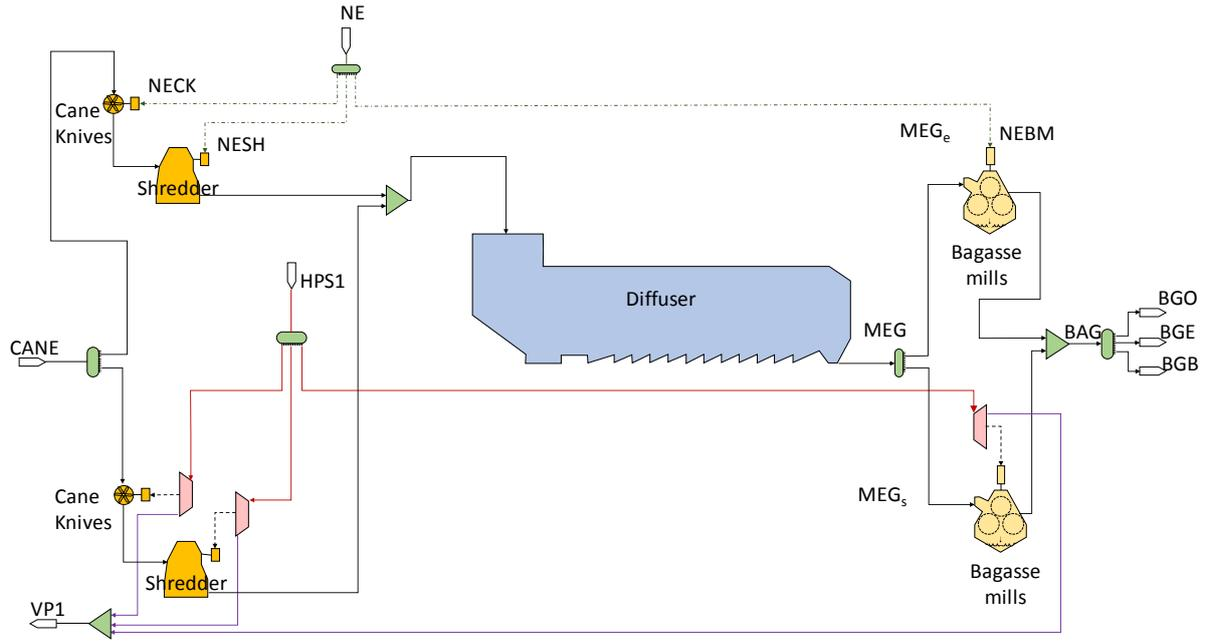
**Figure 1. Visualisation of energy supply to prime movers in the extraction section. Only the process-side flows associated with fibre are shown.**
