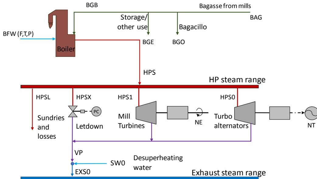
Figure 3. Schematic diagram of the HP steam distribution for the upgraded utilities model.
