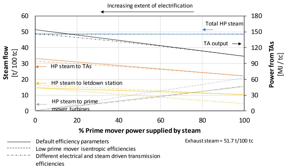
**Figure 4. Simulation outputs using base case model parameters and varying proportion of prime mover power supplied by steam.**
