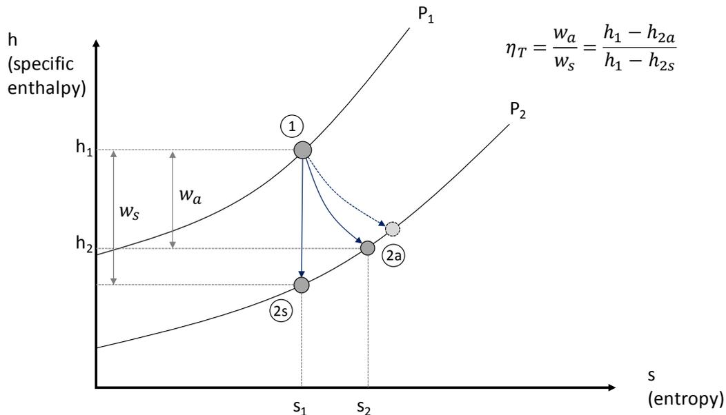
**Figure 5. Enthalpy-entropy diagram for expansion of steam through a back-pressure turbine from pressure  $P_1$  to  $P_2$ .**
