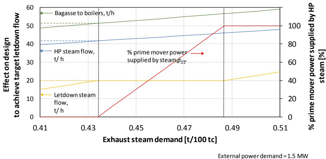
**Figure 7. Effect of factory exhaust steam demand on factory energy demand for a fixed external power demand and a target letdown steam flow rate of 20 t/h. Dashed lines show bagasse and HP steam flow when the design value for letdown steam flow is not permitted to drop below 20 t/h.**
