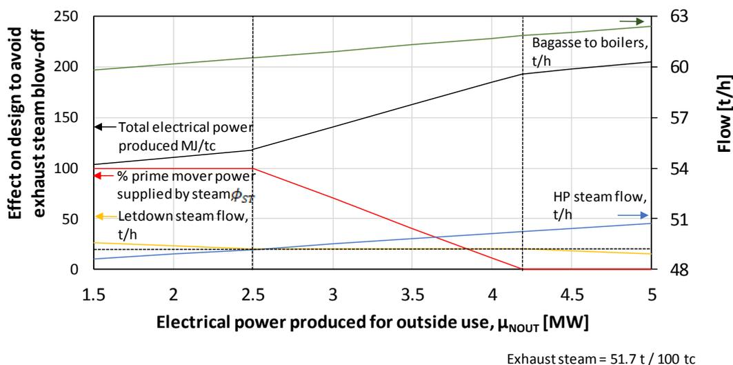
**Figure 6: Effect of increased external power supply on factory energy design for a fixed exhaust steam demand and a target letdown steam flow rate of 20 t/h.**
