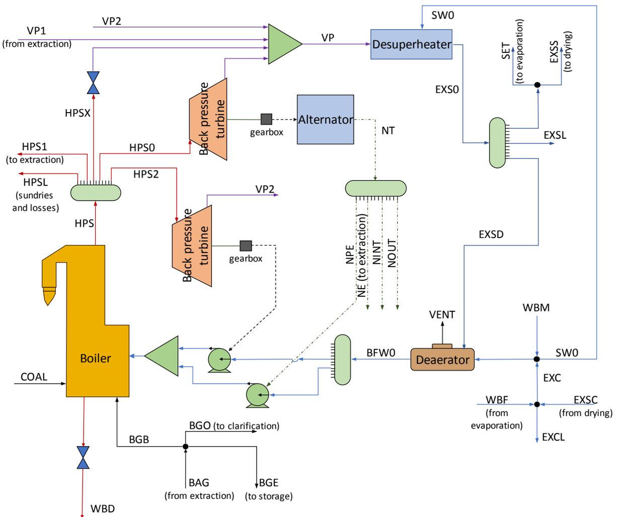
**Figure 2. Steam and power generation and distribution diagram for the upgraded utilities model.**
