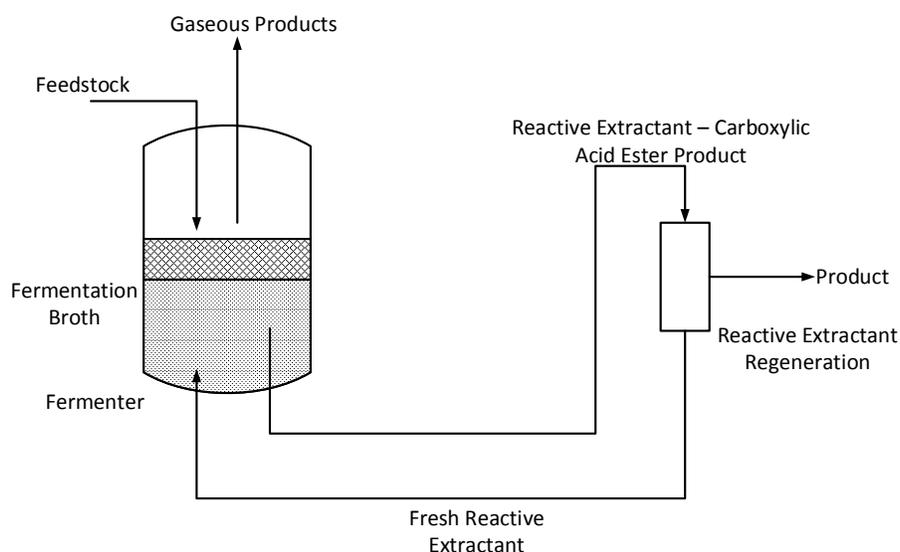
**Figure 1. Simplified process scheme for the reactive extraction of carboxylic acids from fermentation broths.**
