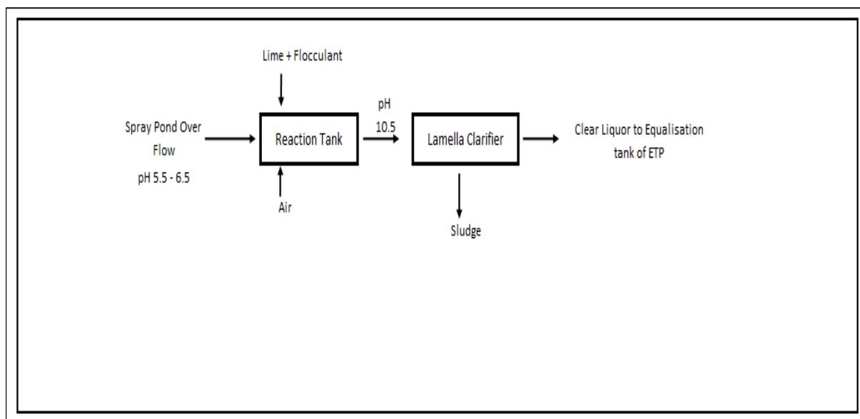
**Figure 4. Spray pond overflow treatment, Trial 1.**
