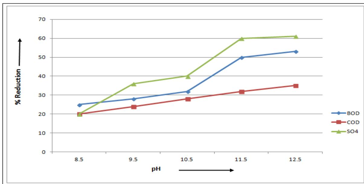
**Figure 3. Percentage reduction in pollutants, viz. biological oxygen demand (BOD), chemical oxygen demand (COD) and sulphate content (SO<sub>4</sub>) by using a lime at different pH (type 2).**
