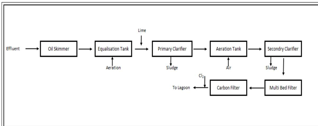
Figure 1. Activated sludge process.
