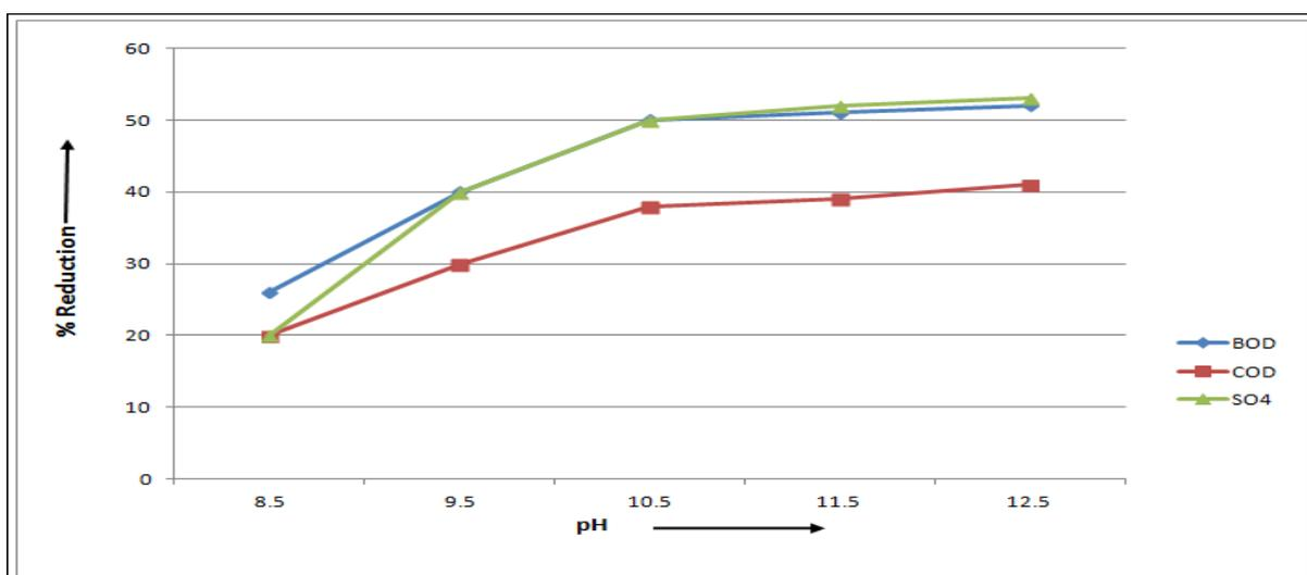
Figure 2. Percentage reduction in pollutants, viz biological oxygen demand (BOD), chemical oxygen demand (COD) and sulphate content (SO<sub>4</sub>) by using a lime at different pH (type 1).
