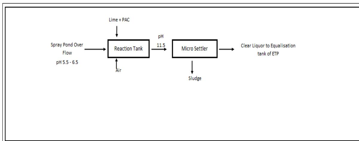
**Figure 5. Spray pond overflow treatment, trial 2.**
