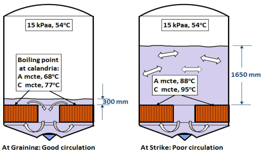
Figure 1. Boiling point is elevated by purity, density and pressure (head).
