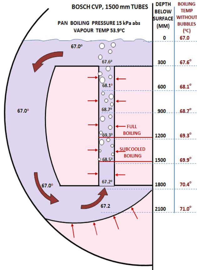
**Figure 5. Boiling in a single tube; temperatures are ignoring the effect of bubbles on boiling point elevation (BPE).**
