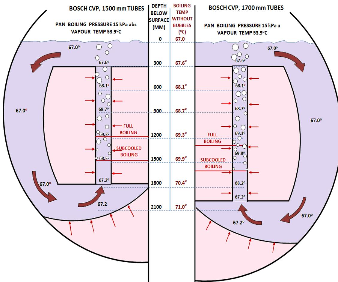
Figure 6. Comparison of boiling in 1500 mm and 1700 mm tubes.
