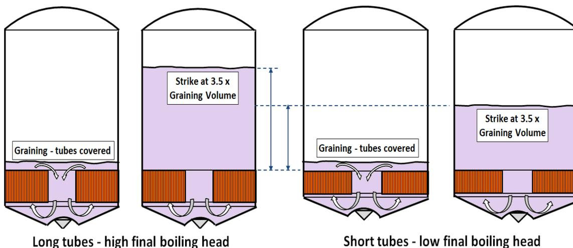
Figure 2. Effect of tube length in batch pans.
