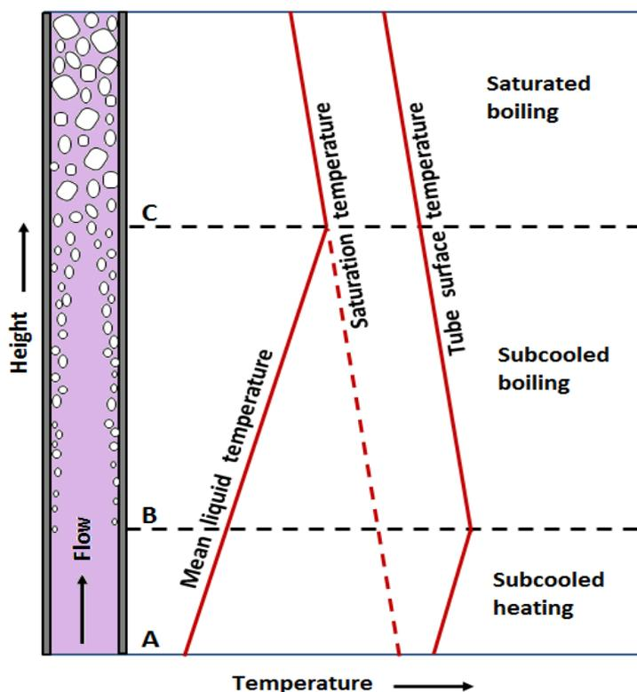
Figure 3. Boiling in a vertical tube (per Rouillard, 1985).
