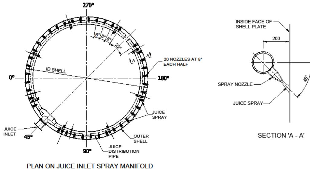
**Figure 3. Arrangement of incoming juice sprayed onto vessel wall.**
