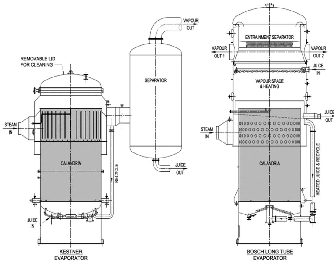
**Figure 2. Kestner and Bosch Long Tube Evaporator with internal clear juice DC heater (both 6 000 m<sup>2</sup> HS).**
