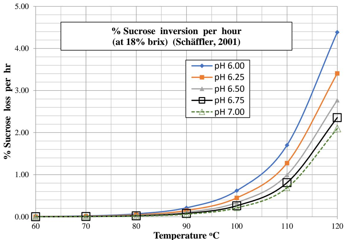
**Figure 1. Sucrose loss per hour at different process conditions using the Vukov formula as per Schäffler (2001).**
