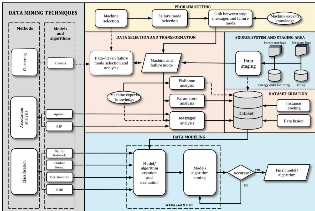
Figure 6. Predictive maintenance conceptual framework (Accorsi *et al.*, 2017).
