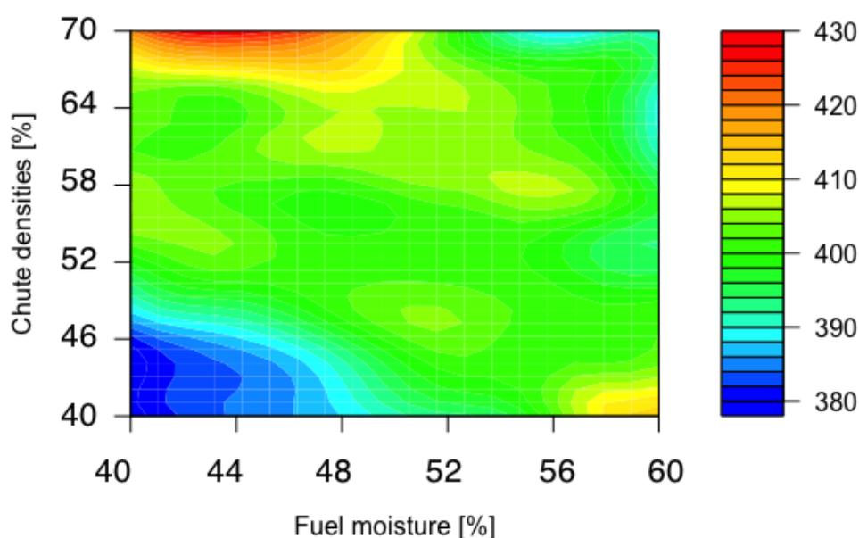
**Figure 4. Artificial Neuron Network (ANN) final steam temperature predictions for varying fuel moisture and fuel density**
