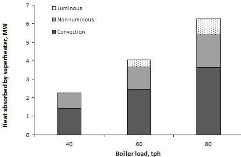
**Figure 4. Different modes of heat transfer for coal firing.**
