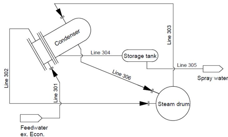
**Figure 8. Integral condenser system.**
