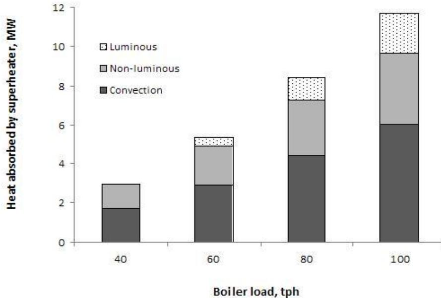
**Figure 3. Different modes of heat transfer for bagasse firing.**
