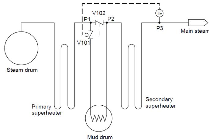
**Figure 6. Mud drum attemperator system.**
