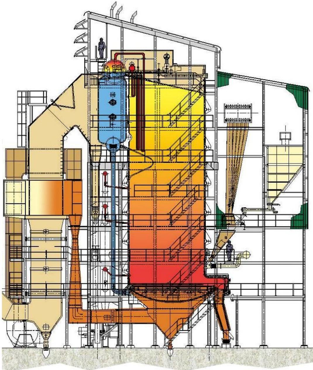
**Figure 2. Boiler with a combination type unscreened superheater.**
