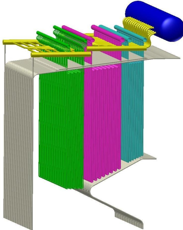
**Figure 1. The top of a furnace showing the platen superheater directly above the furnace and two combination superheater banks above the furnace nose.**
