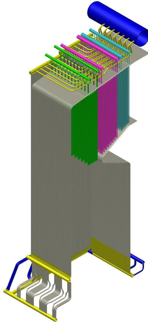
**Figure 5. A three-stage superheater in a monodrum boiler.**
