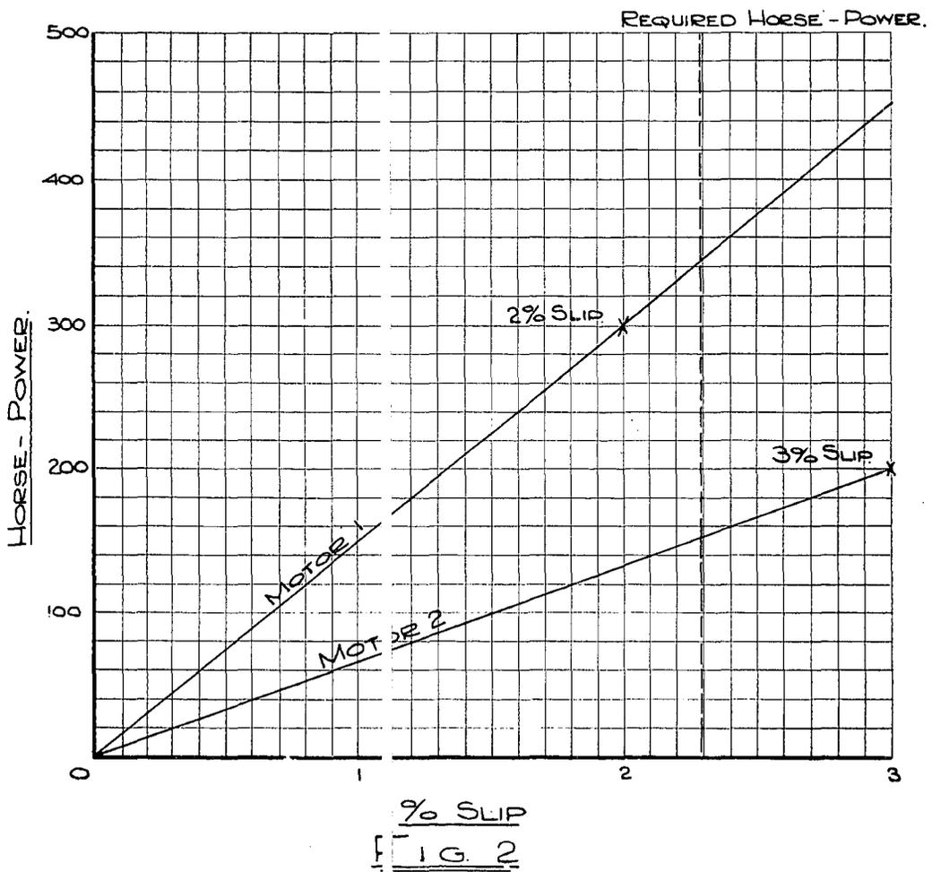
A crude method exists for overcoming the first obstacle. This is to add enough resistance into the rotor circuits of both motors to raise their full load slip to between 5 per cent and 10 per cent, these resistances are then adjusted by trial and error until the motors are matched. This method could waste approximately 28 kw. when applied to both motors in the above example, thus introducing an extra  $7\frac{1}{2}$  per cent loss into the system.
