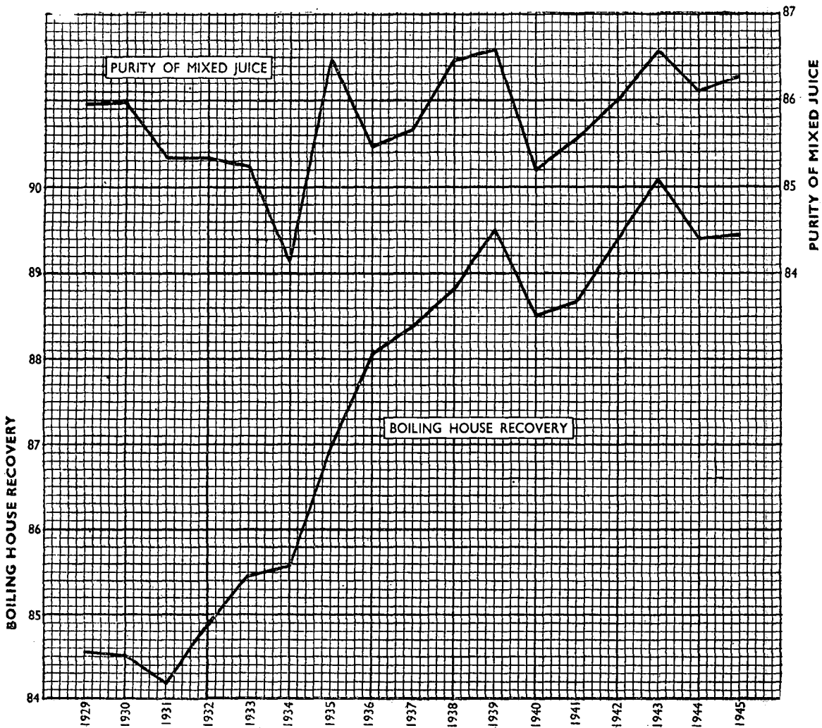
GRAPH B — BOILING HOUSE RECOVERY AND PURITY OF MIXED JUICE ARITHMETICAL AVERAGES FOR 12 FACTORIES, 1929/45
