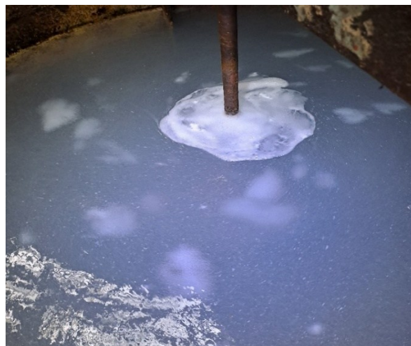
Figure 15. A poorly-agitated flocculant solution in a tank with conglomerates 'fish-eyes'
