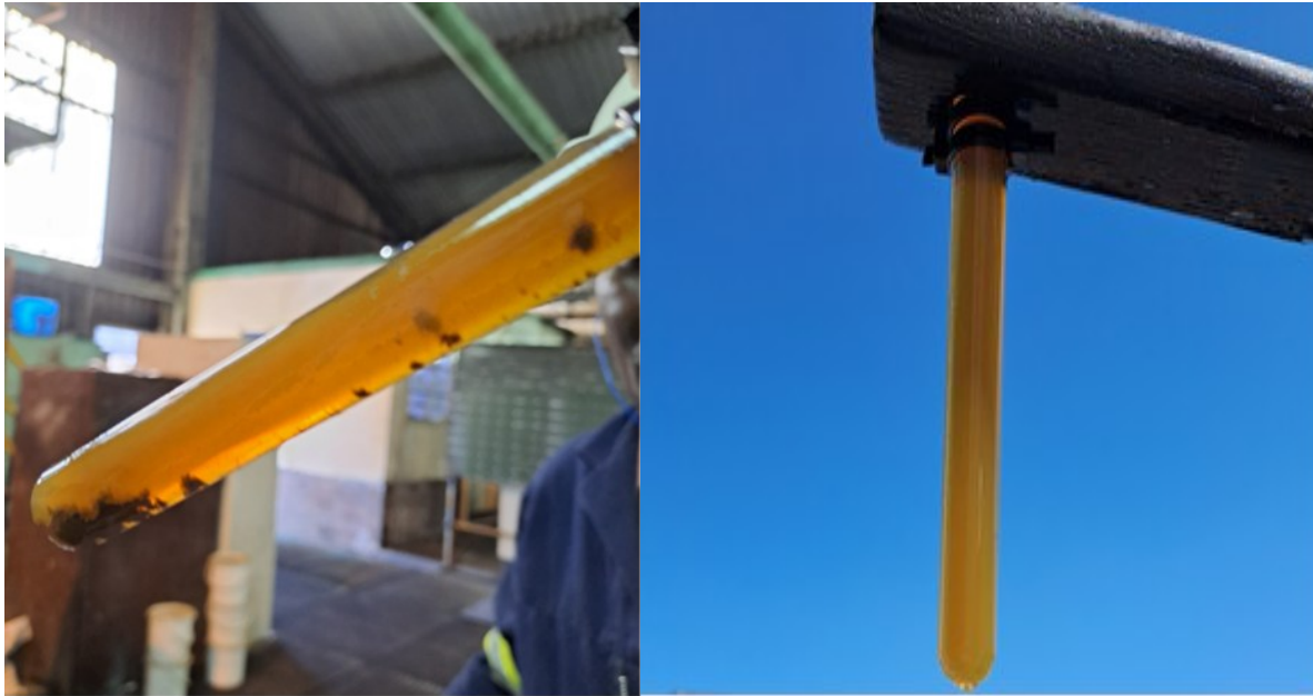
Figure 13. CJ samples indicating poor quality and the improper settling of mud (left) and good quality (right) observed using a test tube in two different factories
