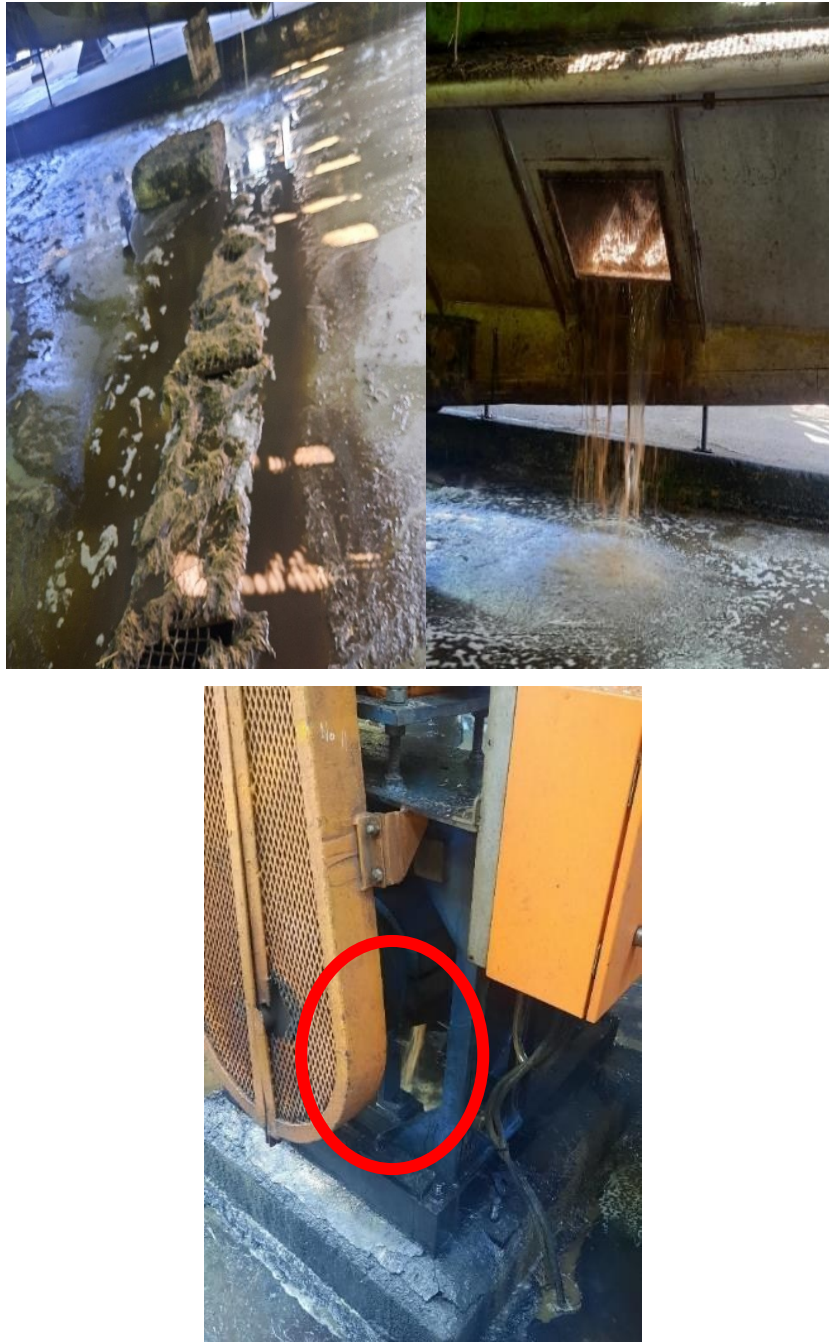
Figure 8. Juice leak from a front-end pump indicated by the red ring. Poor diffuser hygiene observed in factories during the visits
