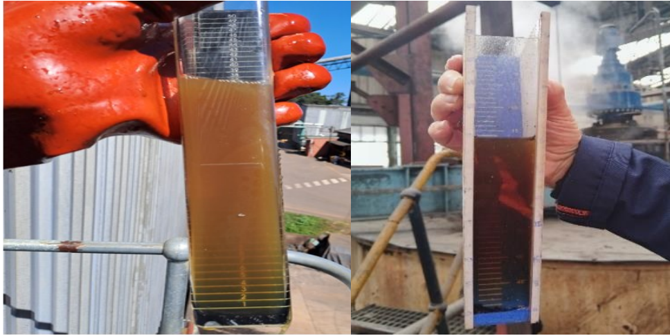
Figure 14. The CJ quality observed using a standard wedge in two different factories, poor (left) and good (right)
