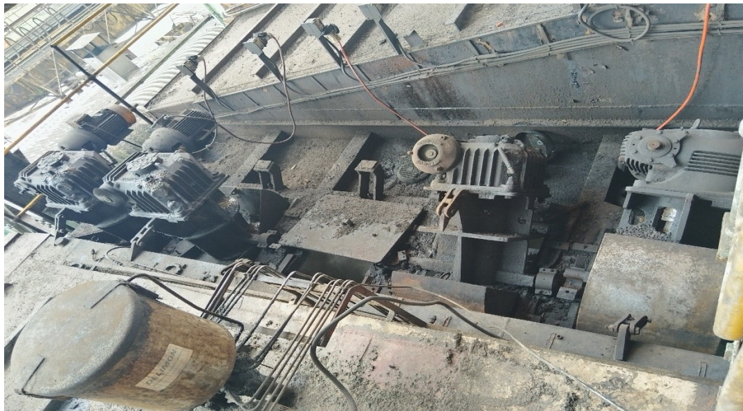
Figure 4. The state of a partly out-of-service set of bed screws, which was a common observation in factories
