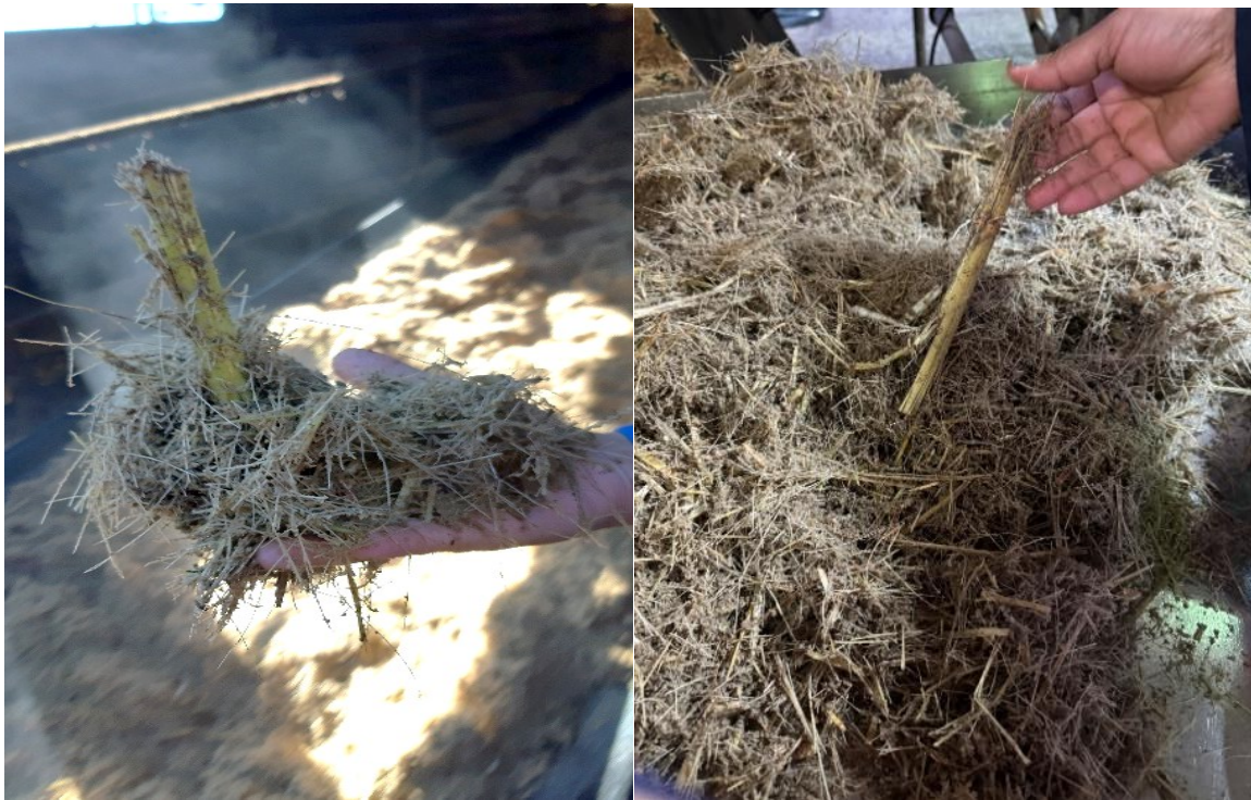
Figure 9. Poorly prepared cane at two different factories
