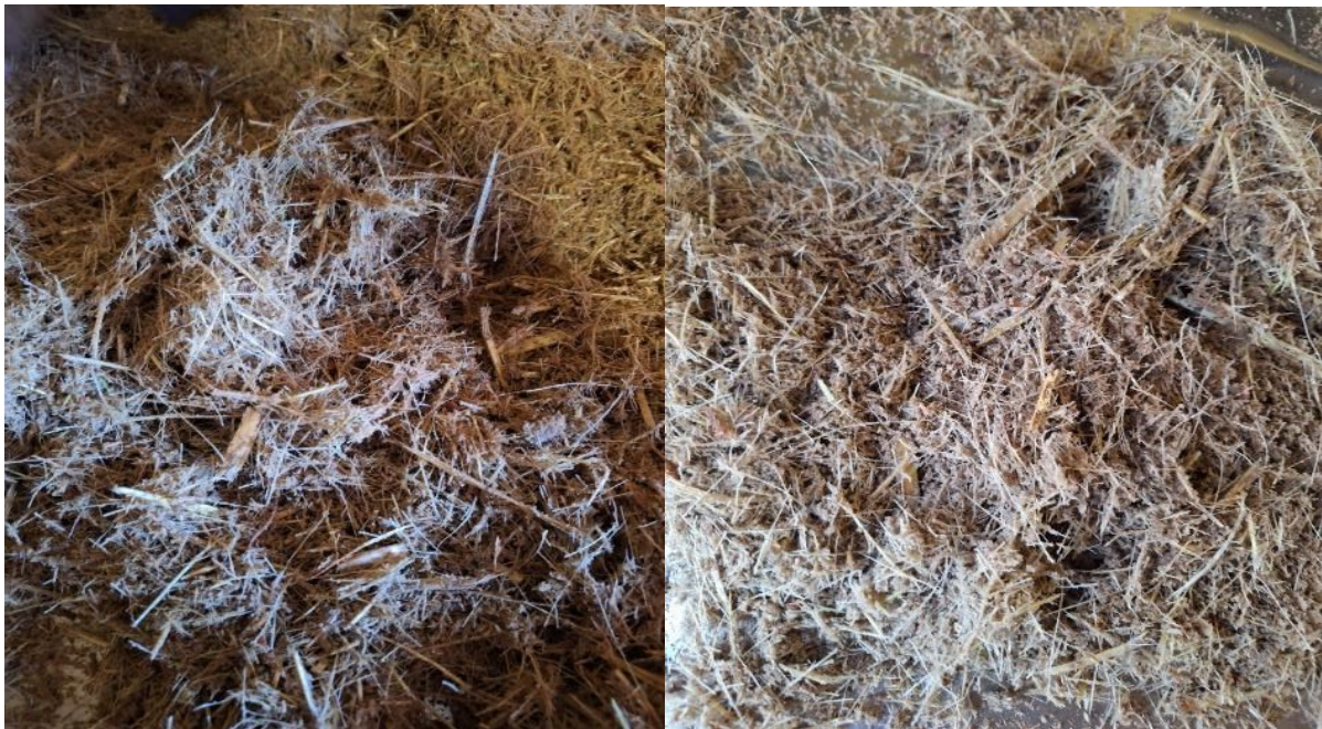
Figure 10. Reasonably well-prepared cane at two different factories
