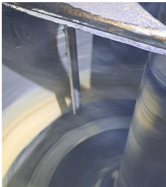
Figure 27. A-Centrifugal – showing sugar left behind after ploughing
