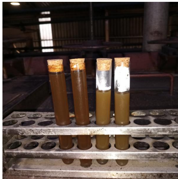
Figure 3. Clear juice from clarifiers (two test tubes on the left) and gravity filtrate (test tubes on the right).
