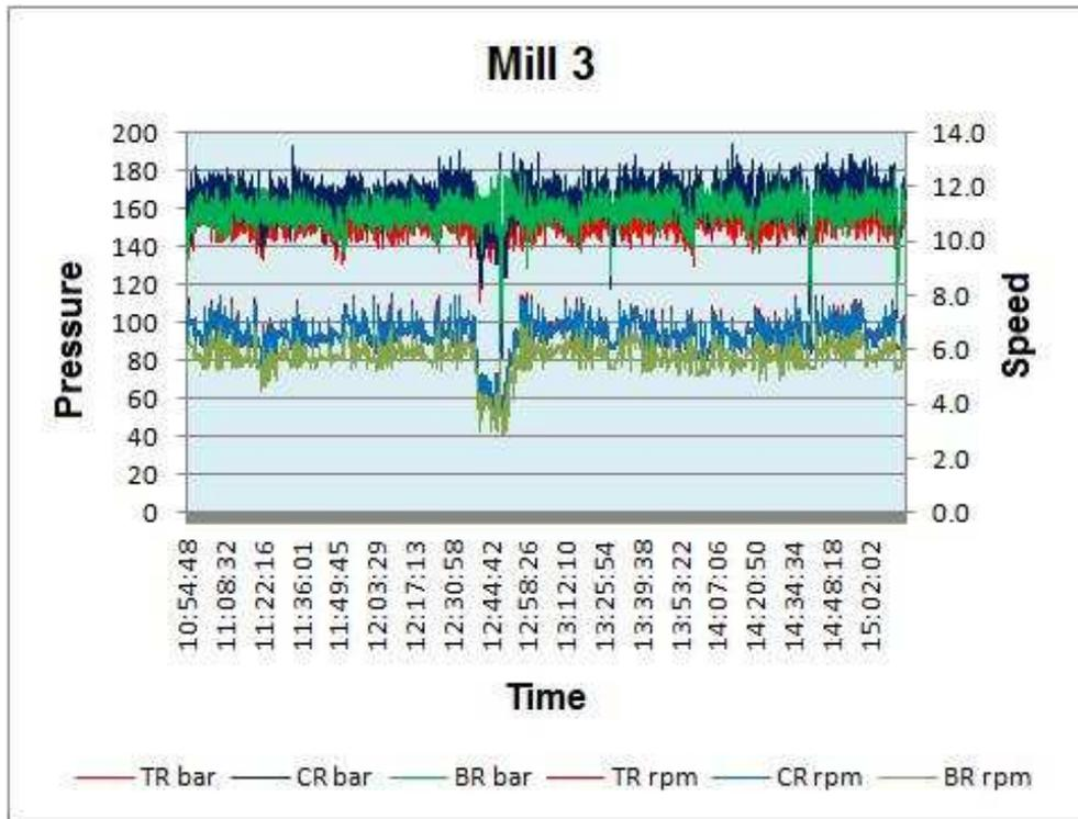
Figure 7c. Mill 3 – Pressure:speed ratio.
