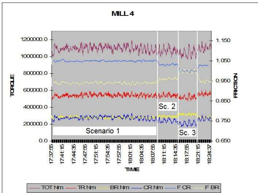
Figure 5b. Mill 4 – Friction:torque ratio.
