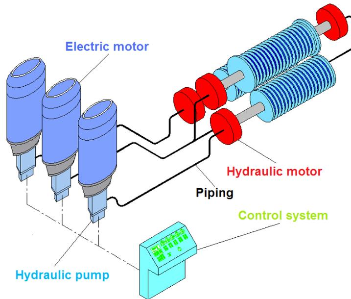
**Figure 1. Individual direct electro hydraulic drive.**
