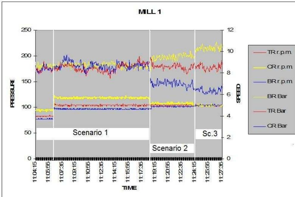
Figure 4a. Mill 1 – Pressure: speed ratio (direct measurement).
