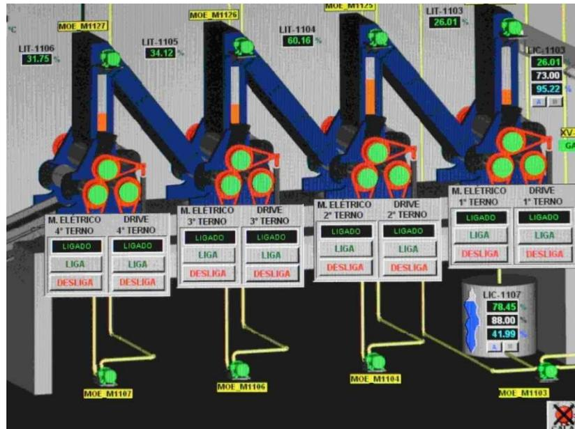
Figure 3. Display of the control system in the Santa Isabel sugar factory.
