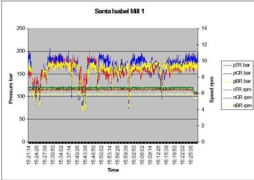
Figure 6a. Mill 1 – Speed:pressure ratio.
