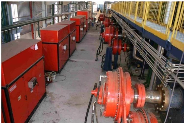
**Figure 2. Milling tandem driven by hydraulic motors in Santa Isabel sugar mill.**
