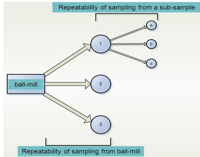
**Figure 3. The method used to evaluate repeatability in sampling (analysis of 1-3), sub-sampling (analysis of a-c) and the use of the Image J<sup>®</sup> technique.**
