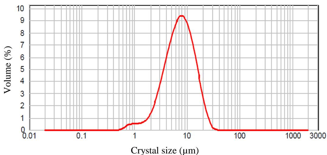
**Figure 1. Laser diffractometry crystal size distribution of a ball-milled slurry.**
