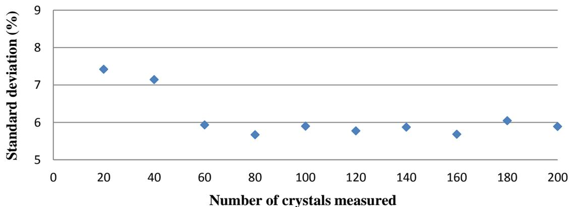
**Figure 2. Standard deviations of slurry crystals as a function of sample size.**
