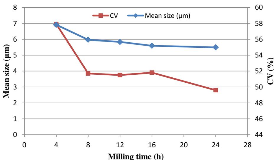
Figure 4. Effect of ball-milling time on mean size and coefficient of variance (CV) of the South African Sugar Technologists' Association prescribed method of slurry preparation.
