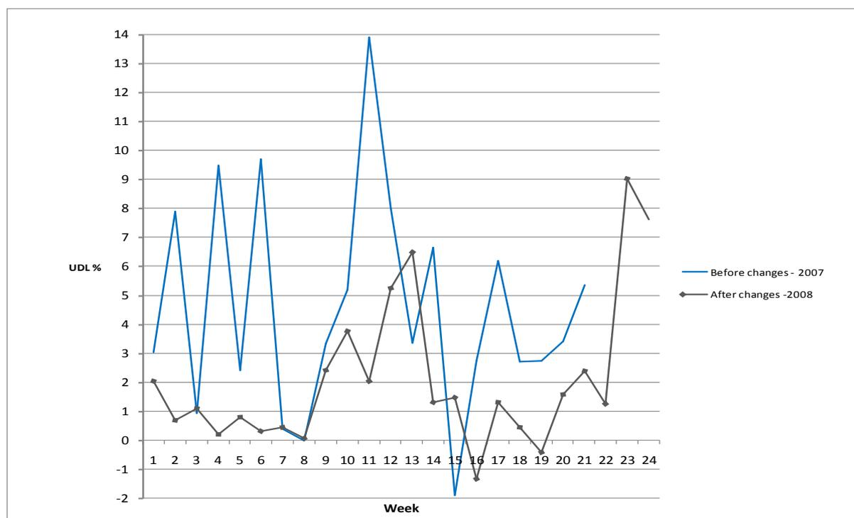
**Figure 5. Undetermined loss (UDL) before and after the four changes made at the Mafambisse mill.**
