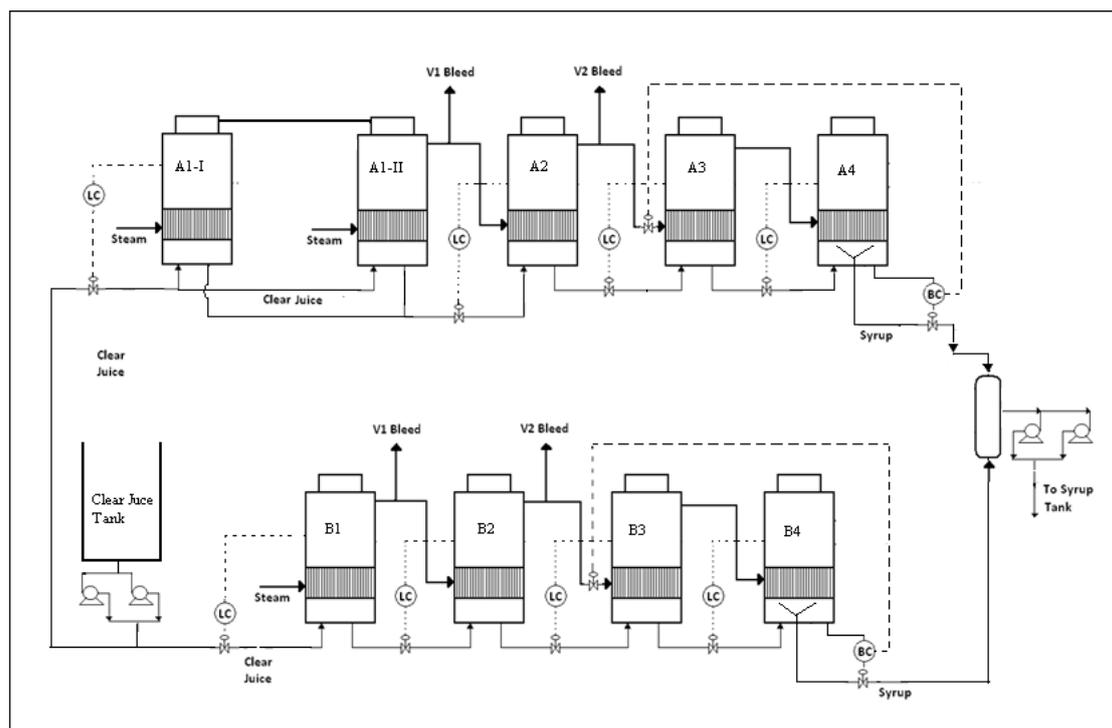
**Figure 3. Evaporator layout before 2008 season with one set of syrup extraction pumps.**
