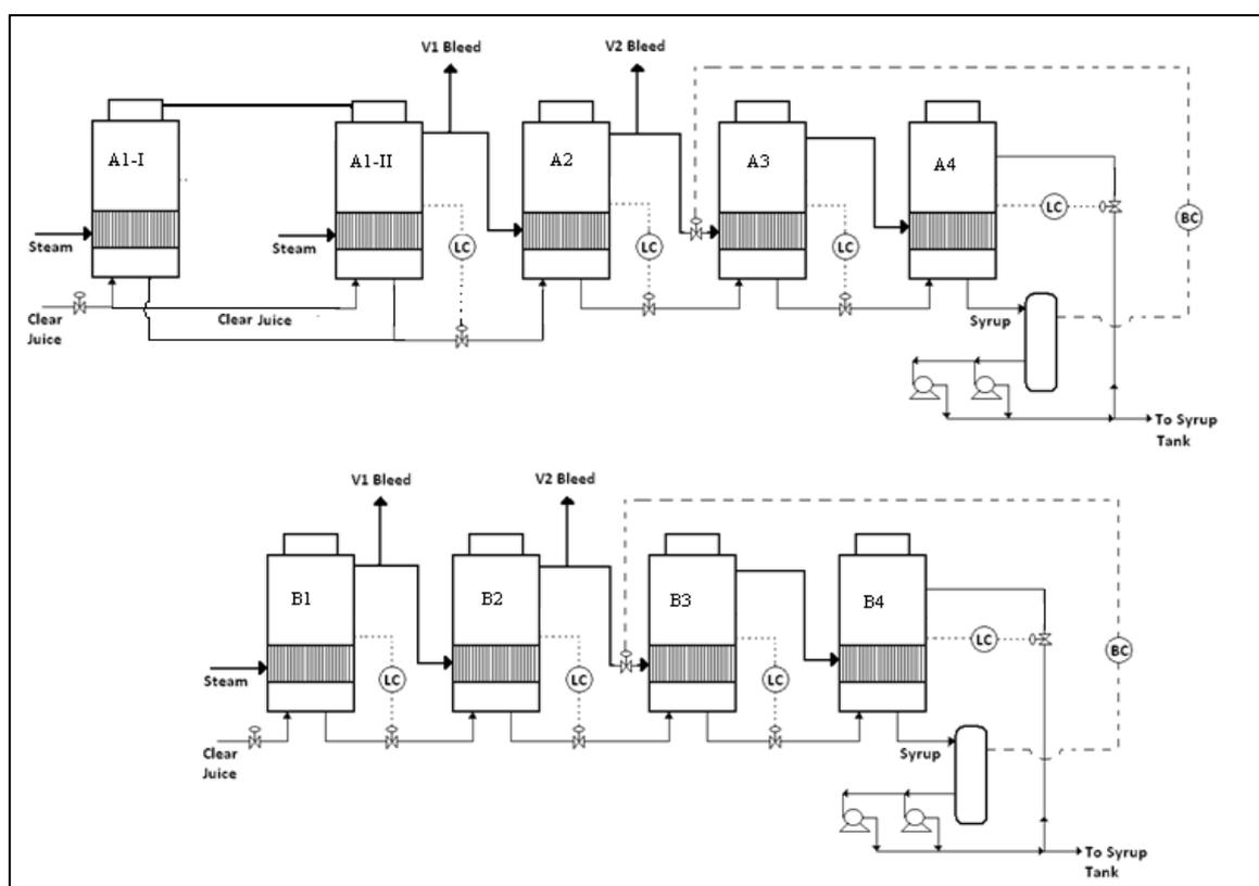
**Figure 4. Modified evaporator layout from 2008 season to include two sets of syrup extraction pumps.**
