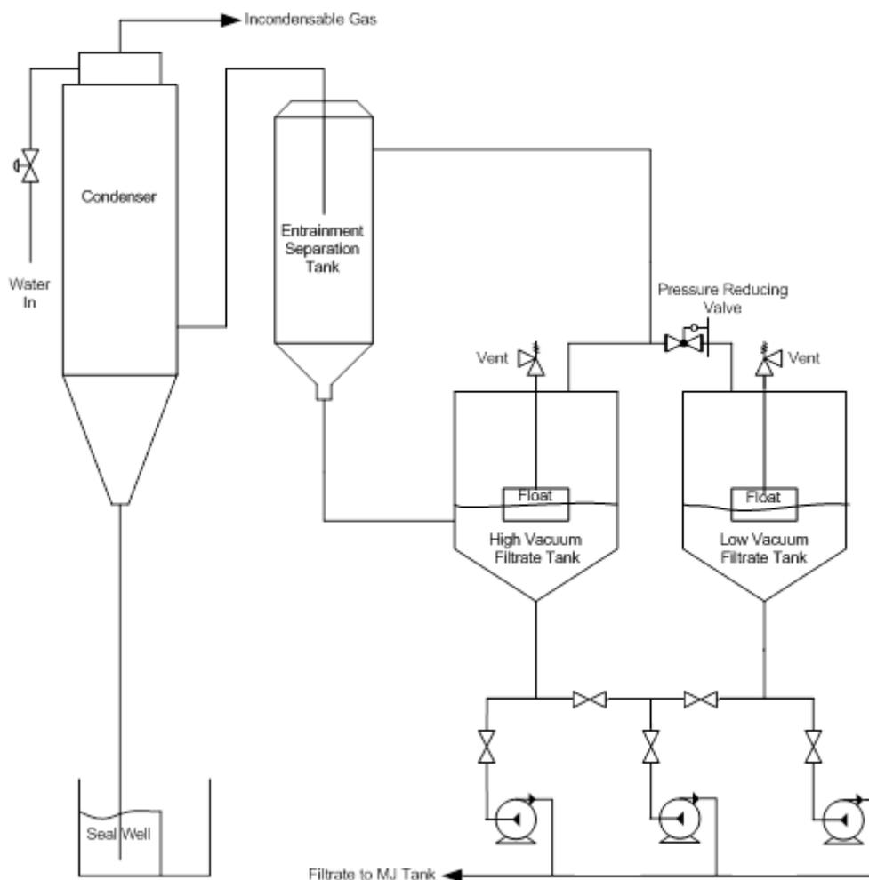
**Figure 1. Original filtrate station layout and control before 2008 season.**
