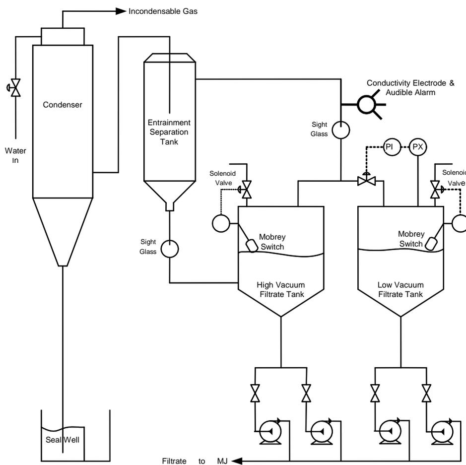
**Figure 2. Modified filtrate station.**
