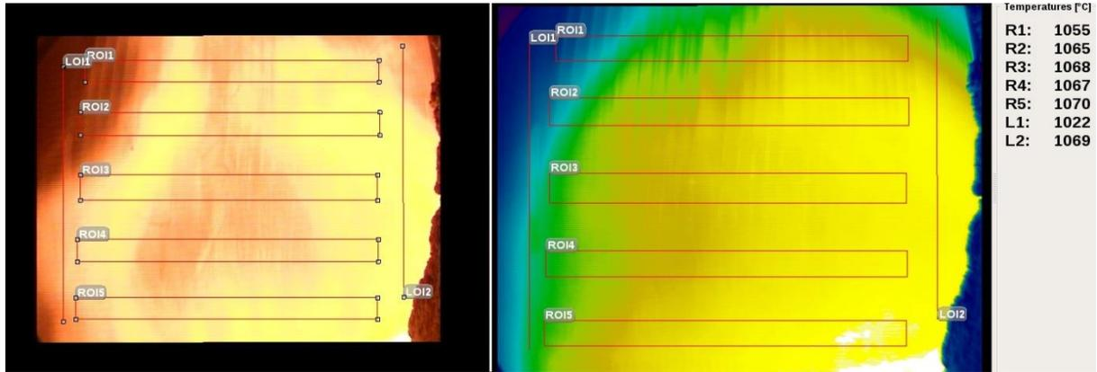
**Figure 8. The actual image of the flame and the superheater on the left and the calculated thermal camera image on the right.**
