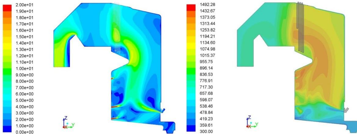
**Figure 3. (a) Velocity contours at the centre of the model (m/s), (b) temperature contours at centre of model (K).**
