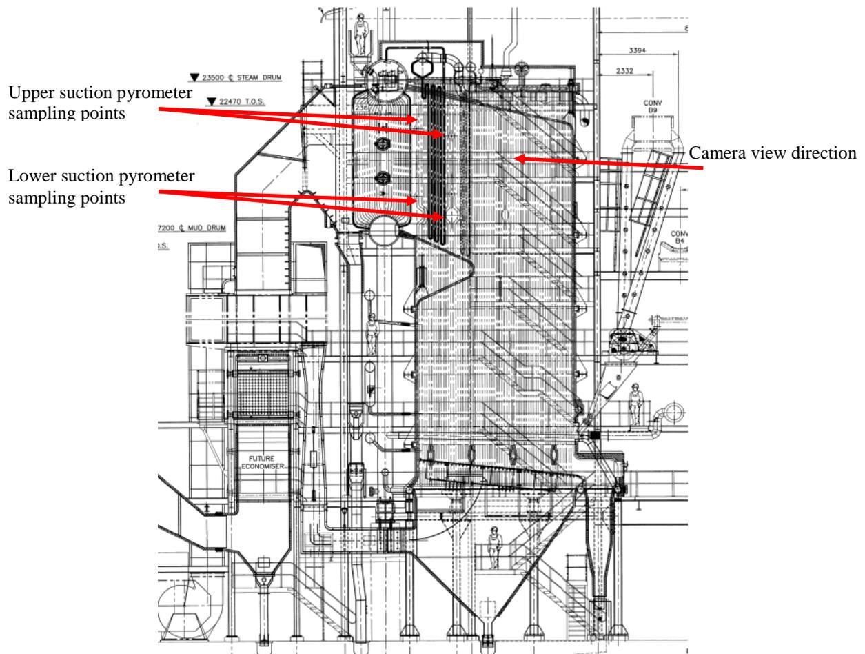
**Figure 5. Positions of suction pyrometer sampling points taken through the width of the boiler and the direction of the camera measurements.**
