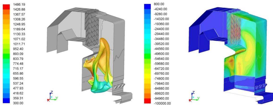
**Figure 4. (a) Iso-surface of the flame profile and temperature (K), (b) heat absorbed through walls (W/m<sup>2</sup>).**
