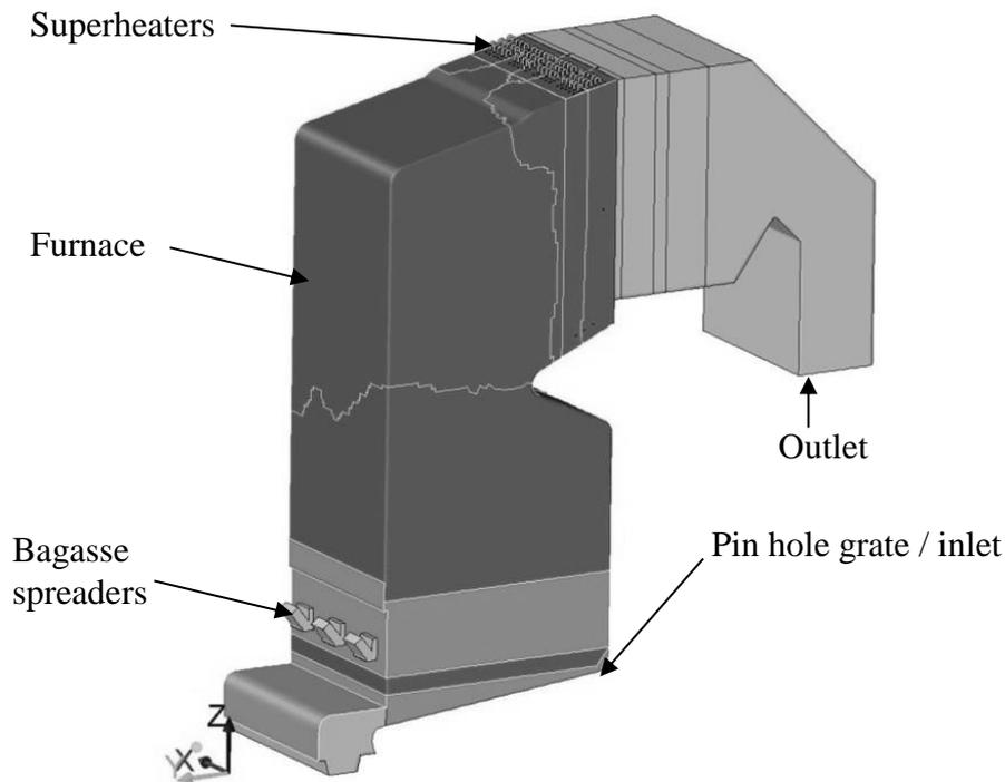
**Figure 1. Diagrammatic view of three-dimensional model of boiler.**
