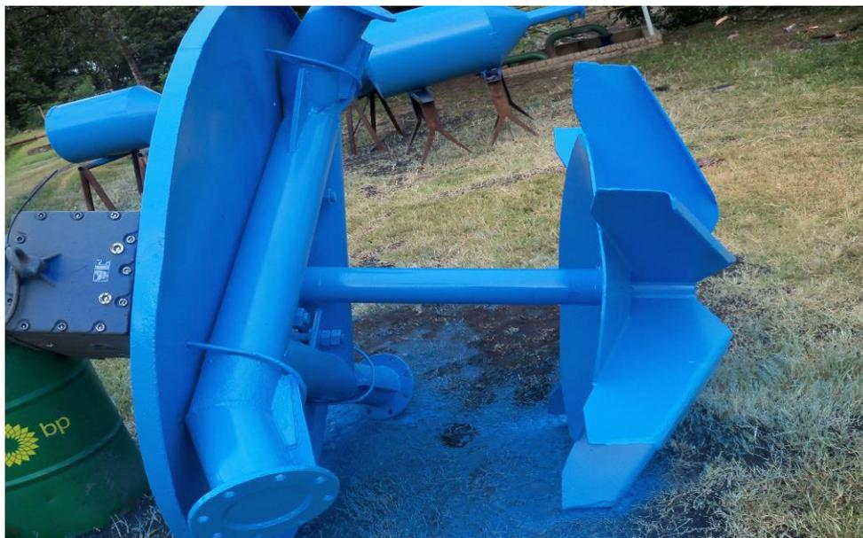
**Figure 11. Refurbished aerator from the aeration pond.**
