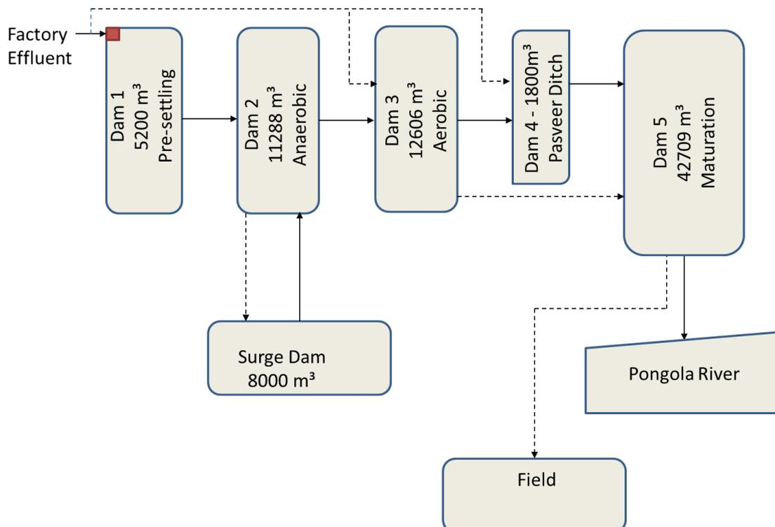
Figure 1: Layout of Pongola mill effluent treatment plant.
