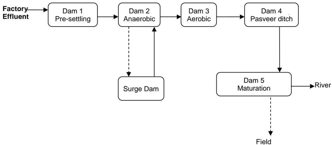
**Figure 8. ETP old effluent flows from Dams 1 to 5.**
