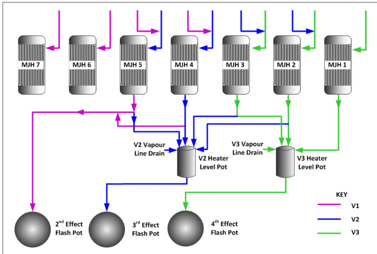
**Figure 2. Dedicated level pot condensate drainage system.**
