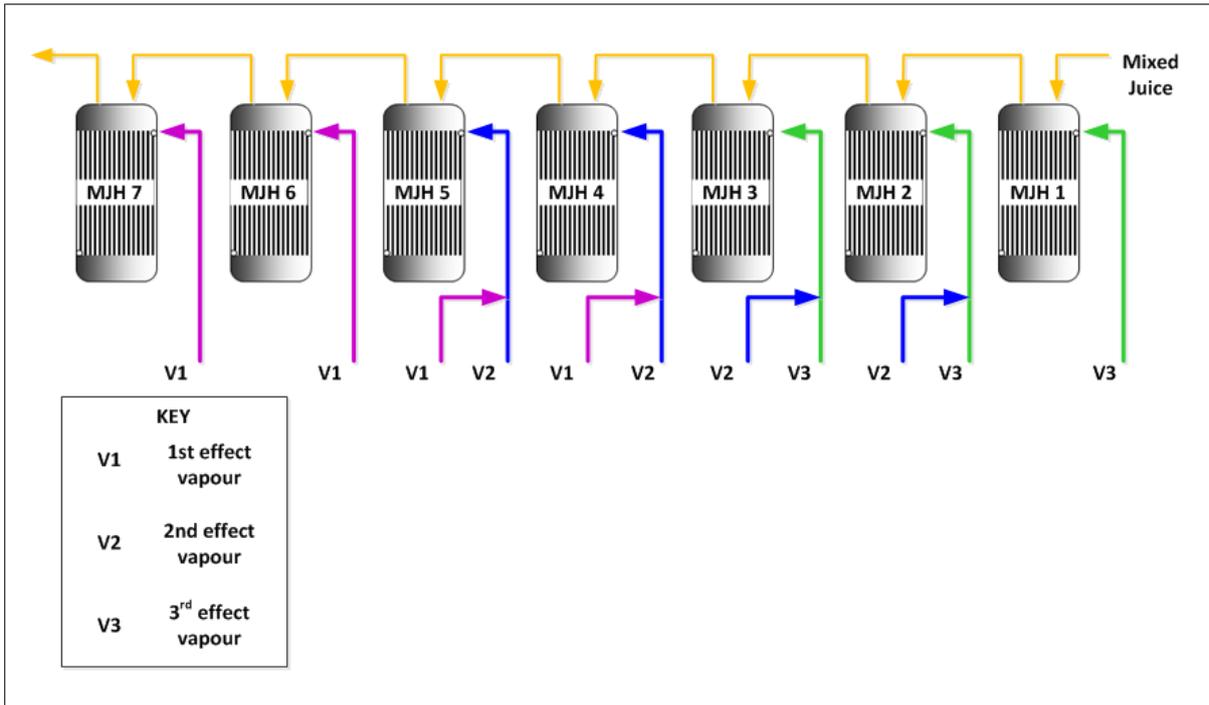
Figure 1. Available vapours for the mixed juice heaters.
