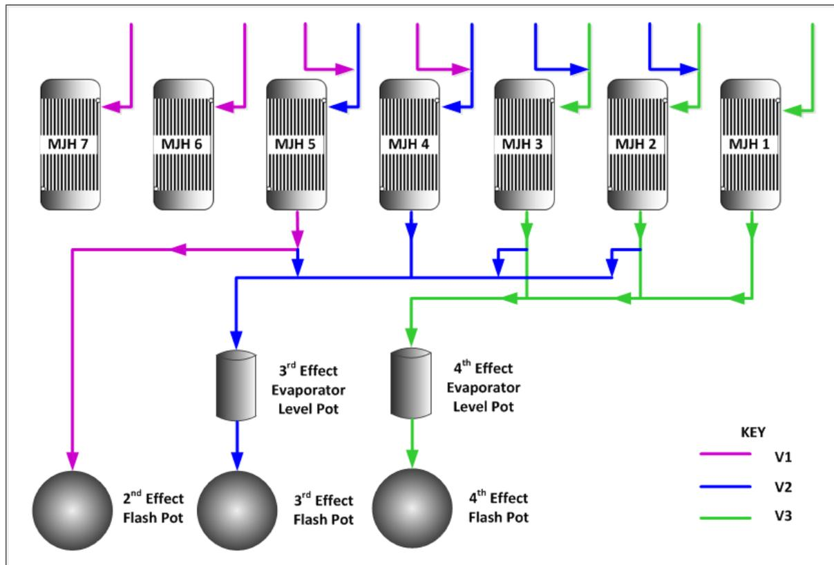
**Figure 1. Manifold type condensate drainage system.**
