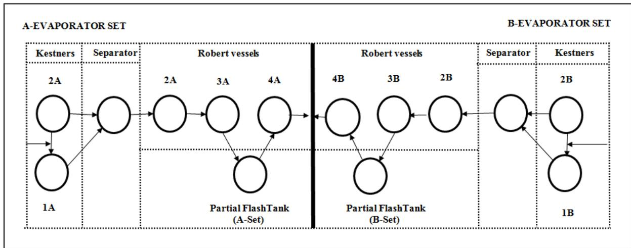
**Figure 5. Modified plan view of set-up showing positioning of partial flash tanks.**
