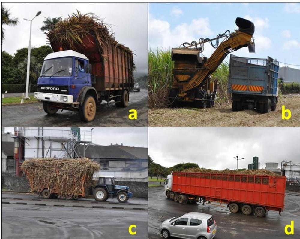
**Figure 1. Four vehicle types used for dispatch optimisation at the FUEL consolidated sugar mill, viz. (a) 15 ton, (b) 18 ton, (c) 6 ton and (d) 33 ton.**
