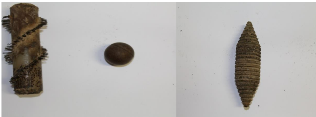
Figure 9. Objects after the trial showing scale deposits.
