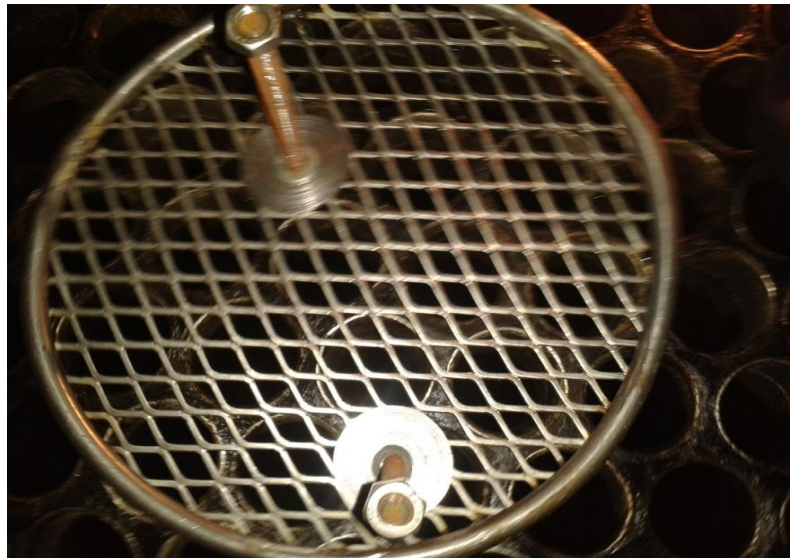
Figure 2. Wire mesh mounted on top of an evaporator tube plate.
