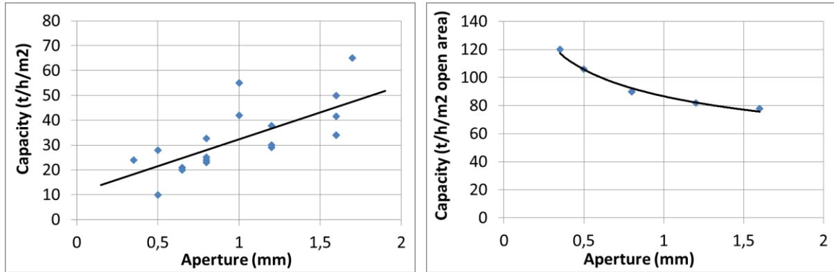
**Figure 2. Wedge wire screen capacities as a function of screen aperture, showing data from Brotherton and Noble (1982) and Manson and Ames (1982)**
