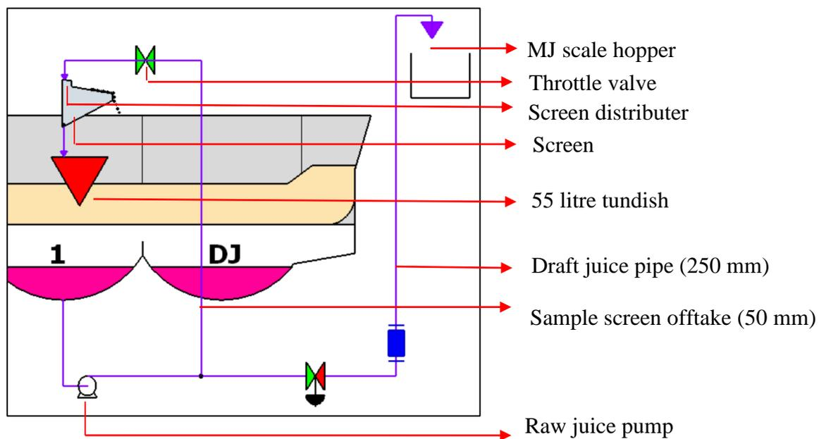
Figure 6: DCJ juice screening trial layout
