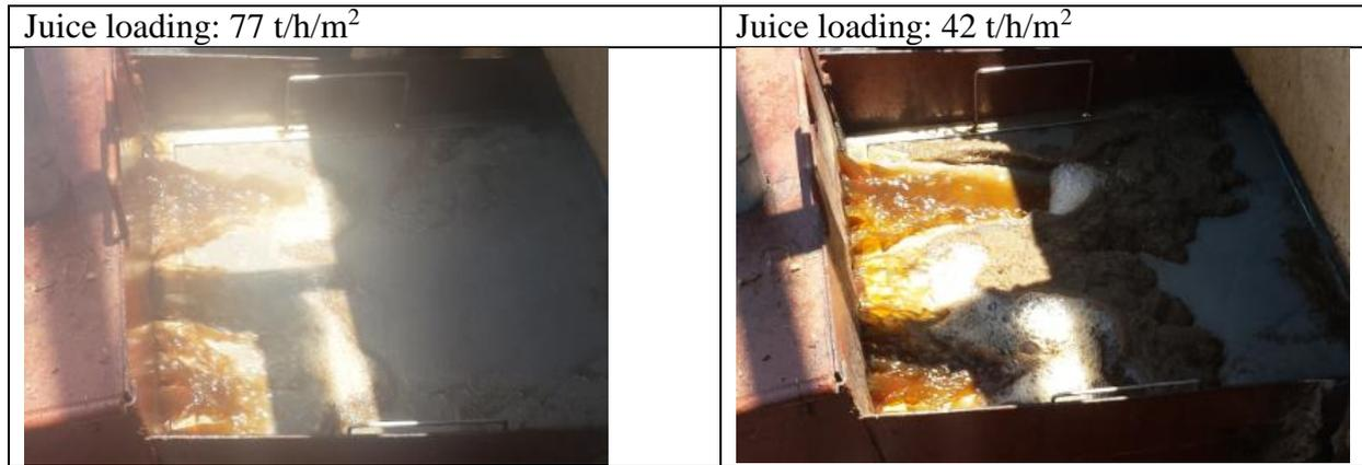
**Figure 7: Juice flowing through sample screen**
