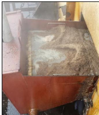
**Figure 11: Fibre build-up on the sample screen**
