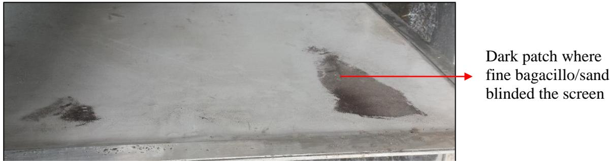
**Figure 12: Woven screen after rinsing off bagasse after ~24h operation with uneven juice distribution onto the screen**
