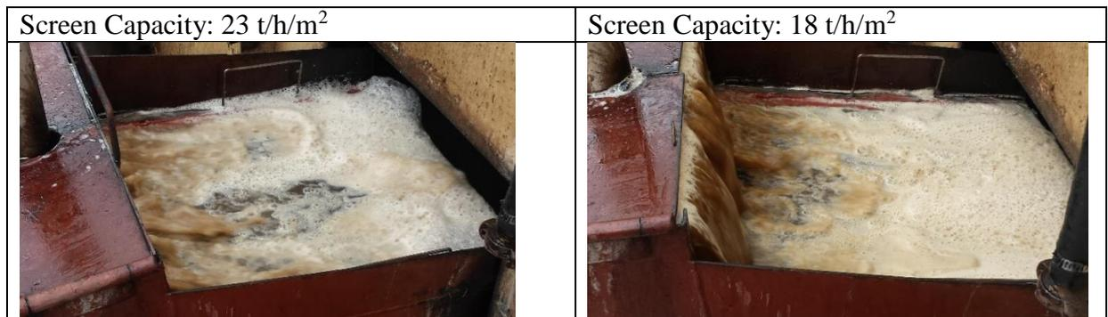
**Figure 8: Maximum juice loading achieved with foaming**
