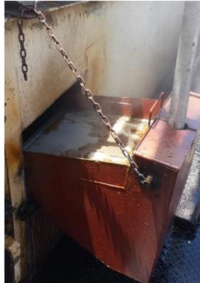
**Figure 10: Trial screen positioned at an  $11^\circ$  screening angle**
