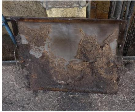
**Figure 9: Vertical screen showing high friction between bagasse and mesh**
