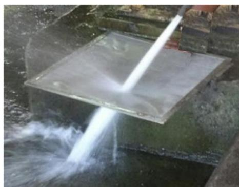
**Figure 4. Pressurised water penetration through a 0.08 mm aperture, 35% open area woven mesh screen**
