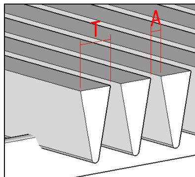
**Figure 1. Wedge wire screen using wire of thickness (T) and aperture (A)**
