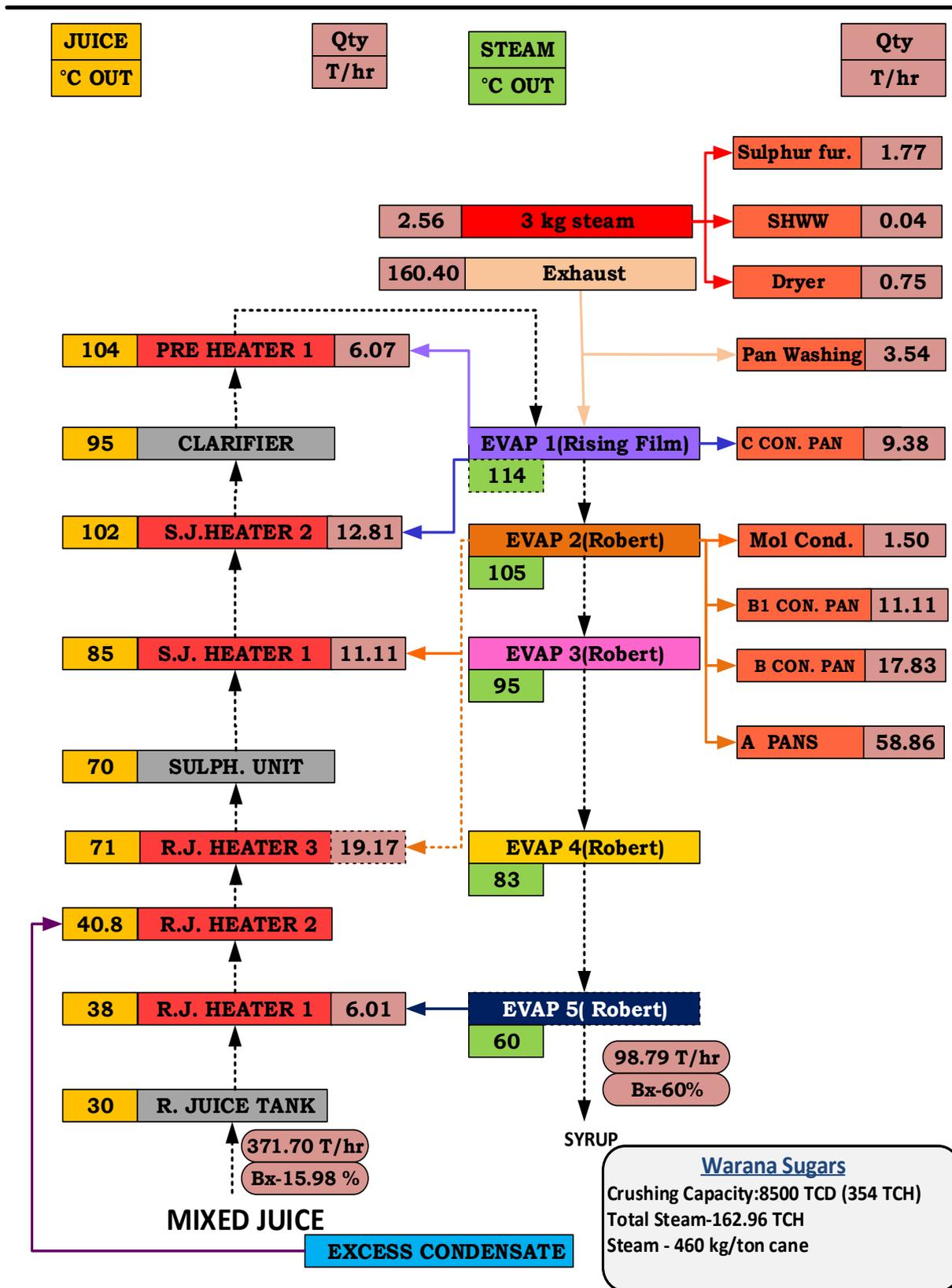
Figure 1. Existing heat and mass balance
