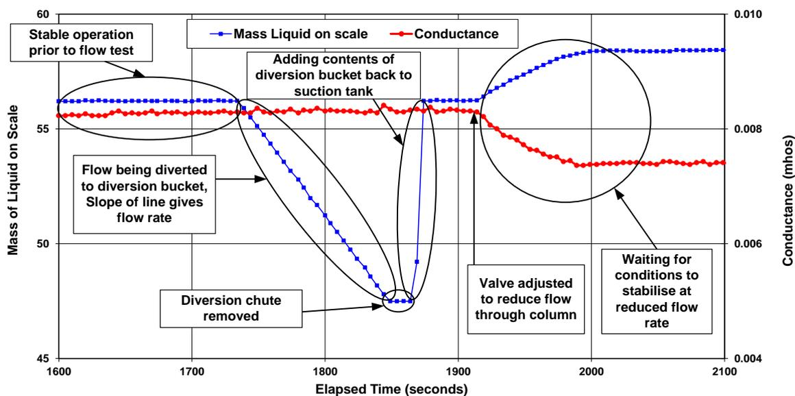
Figure 4. Segment of test run explaining details of a flow test
