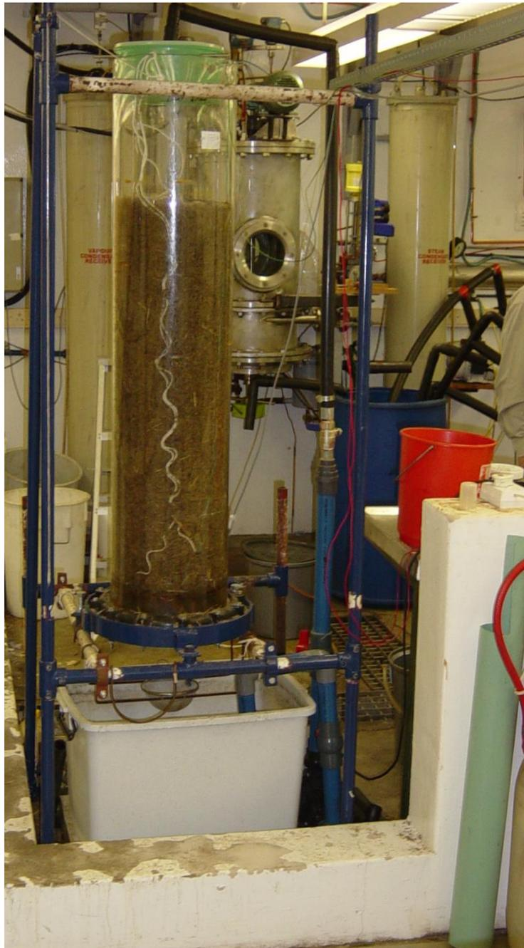
**Figure 1. Batch diffuser column used for laboratory testing**
