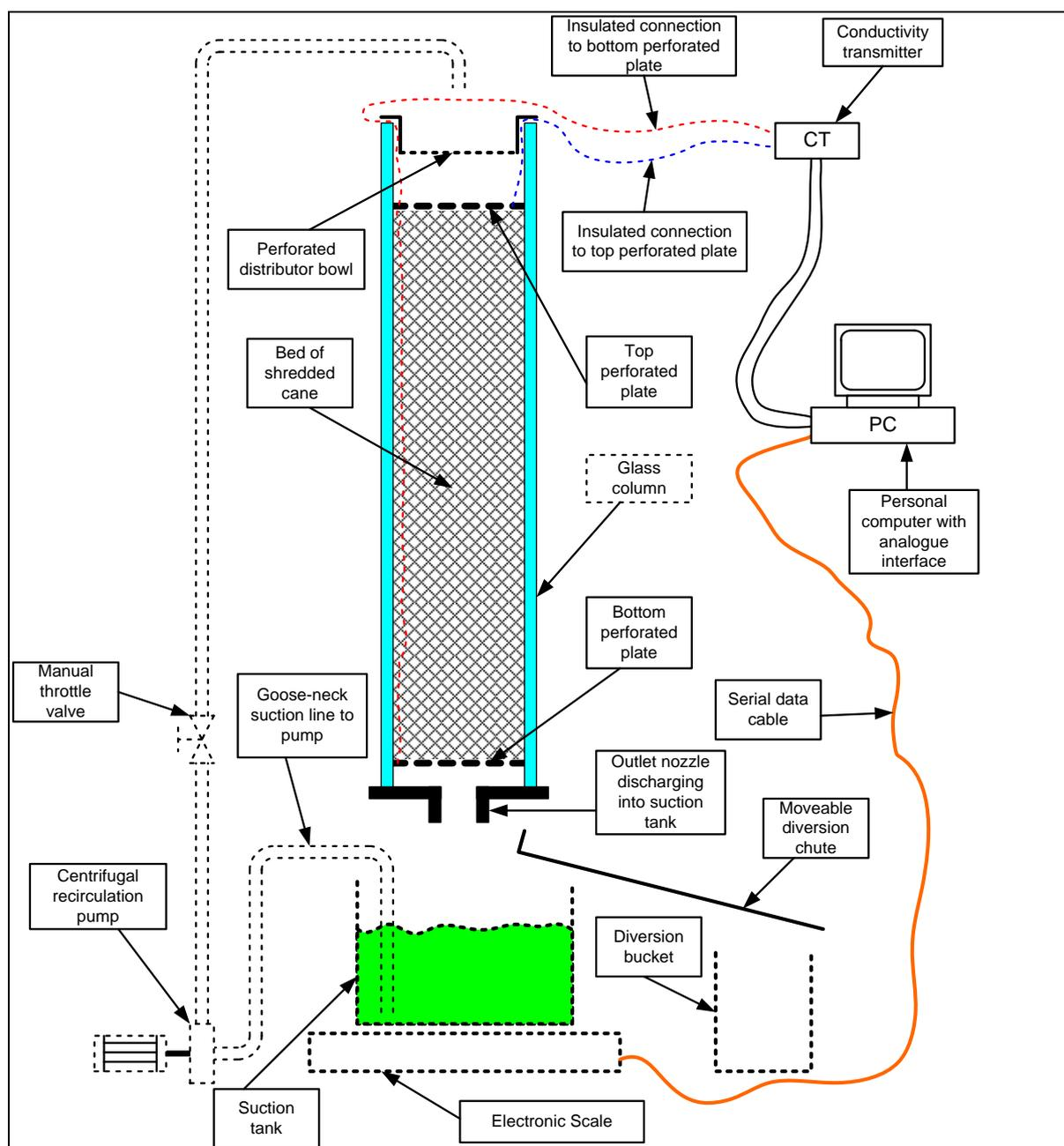
**Figure 2. Schematic diagram of diffuser column and its associated instrumentation**
