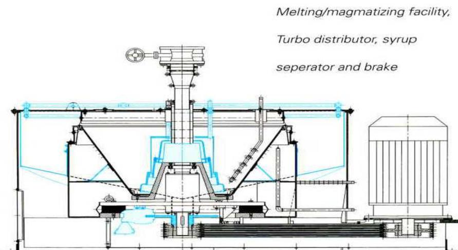
**Figure 1. Schematic drawing of BMA k2300r continuous centrifugal.**
