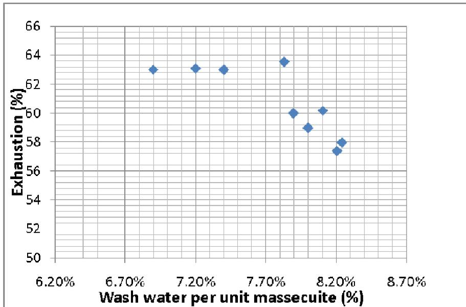
Figure 7. A-exhaustion as a function of wash % massecuite.
