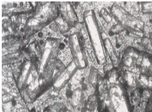
**Figure 3. Crystal elongation present in the sugar used for remelt**
