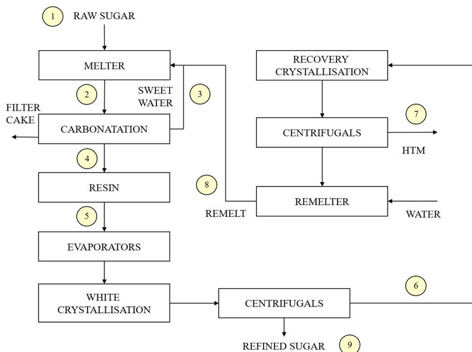
**Figure 2. Basic process flow diagram of the Tongaat-Hulett refinery and sampling points used in the study. Numbers refer to sampling points as referenced in Table 1.**
