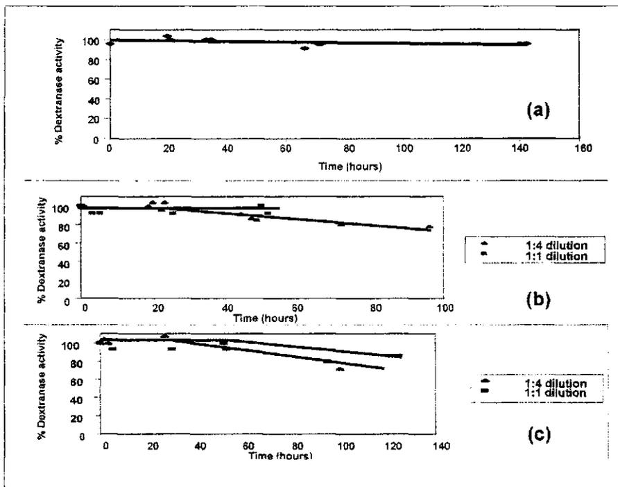
**Figure 4a. Effect of applying a 2-fold working solution of "concentrated" dextranase (52,000 DU/ml) at the factory on 4 Nov, 2004. Conditions: 6 ppm; ~90 °F (32.2 °C)**
