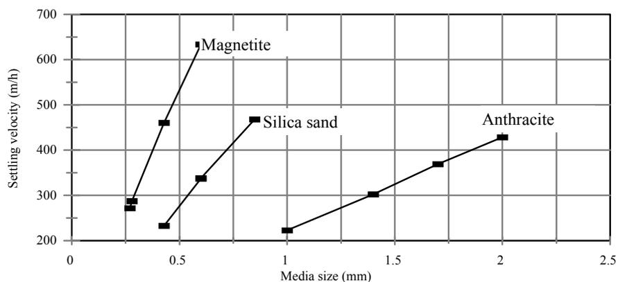
**Figure 3. Settling velocity selection chart for different media used in the deep bed filter.**
