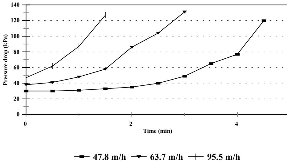
Figure 10. Effect of flow rate on 1.2 g/L feed for coarser media.
