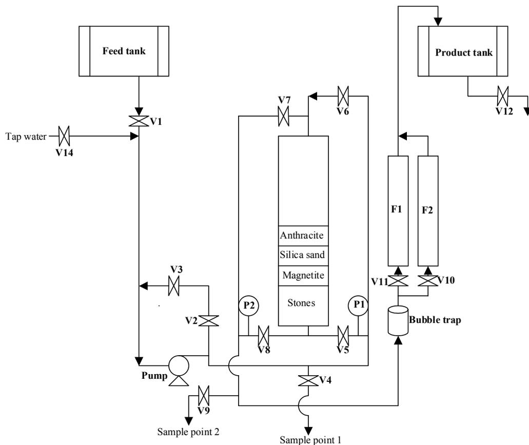
Figure 2. Schematic diagram of the DBF pilot plant.
