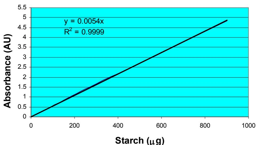
**Figure 1. The Basic Starch Test calibration curve.**
