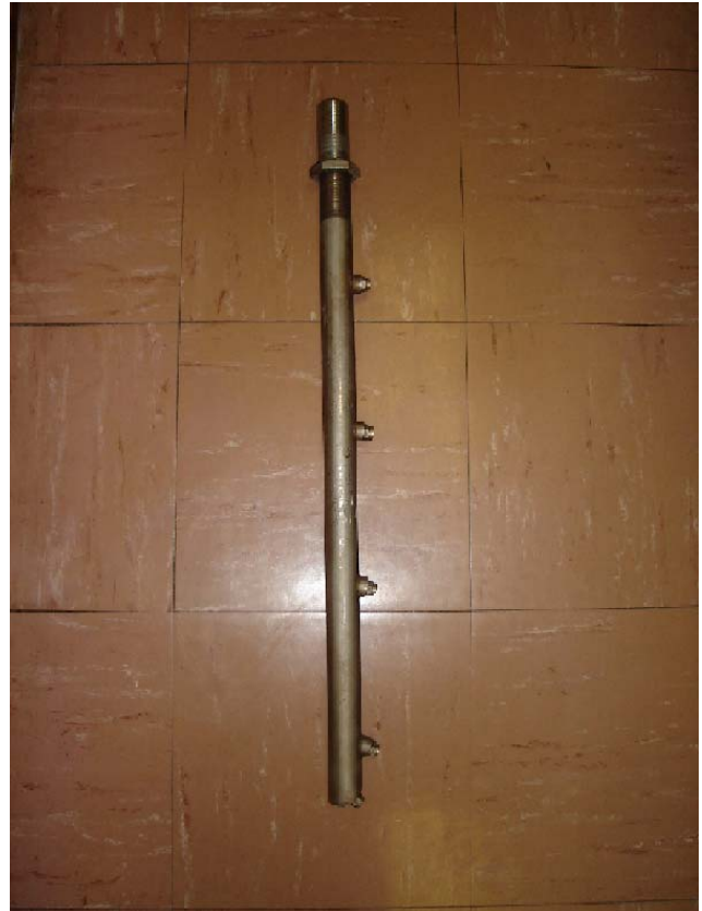
Figure 2. Spray bar with five flat spray nozzles.
