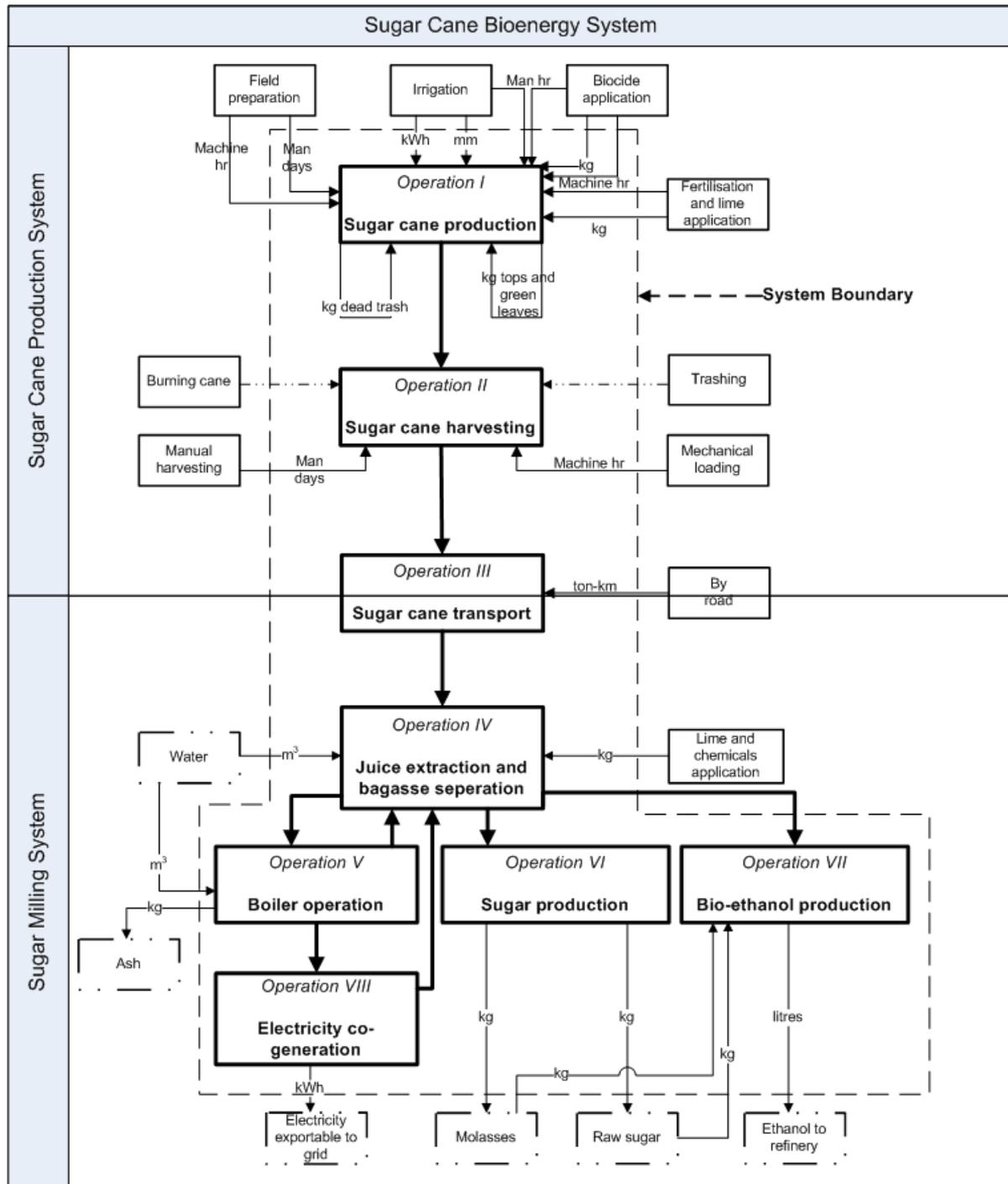
**Figure 1. The sugarcane bioenergy system.**
