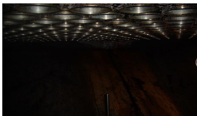
**Figure 9: Condensate trail on AK batch pan 1 saucer.**
