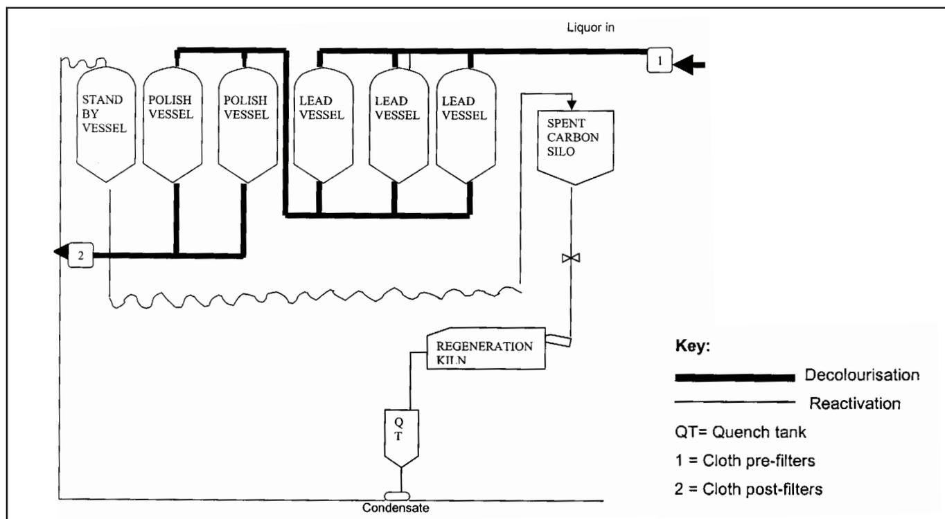
Figure 2. Schematic diagram of the granular activated carbon plant showing the decolourisation and reactivation operations.
