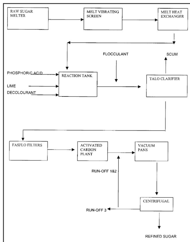
Figure 1. A simplified flow diagram of the Nchalo refinery.
