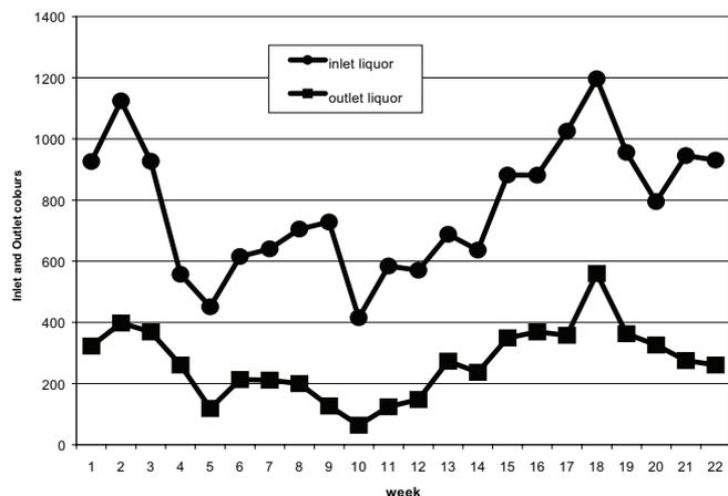
Figure 3. Inlet and outlet colours for the GAC plant.
