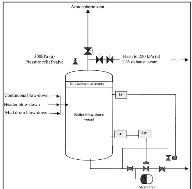
Figure 2. Malelane mill boiler blow-down PFD .
