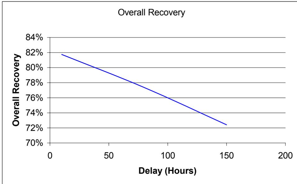
**Figure 2. Effect of cane delay on overall recovery.**
