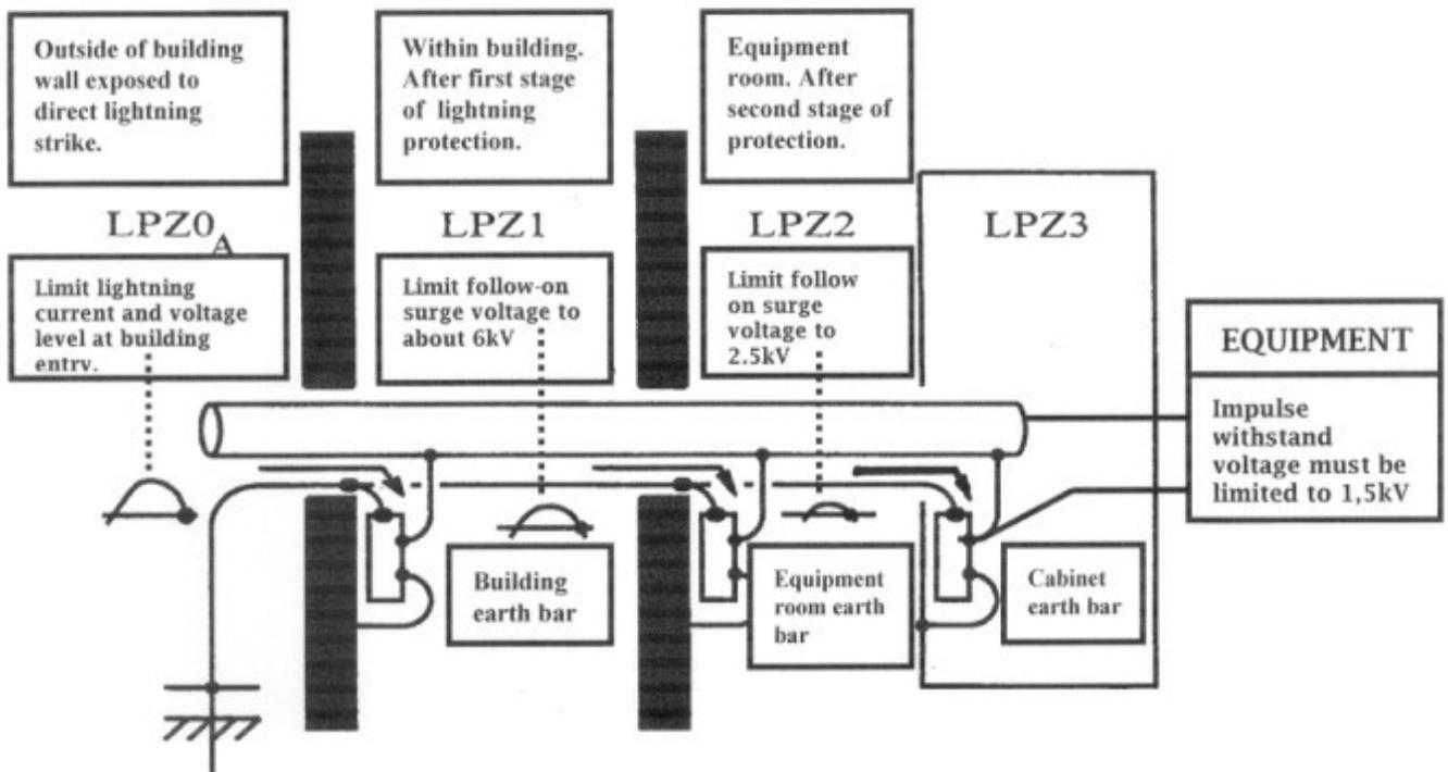
**Figure 3. Systematic protection using the building shielding and co-ordinated surge protection devices to limit the level of surge voltages penetrating into equipment.**
