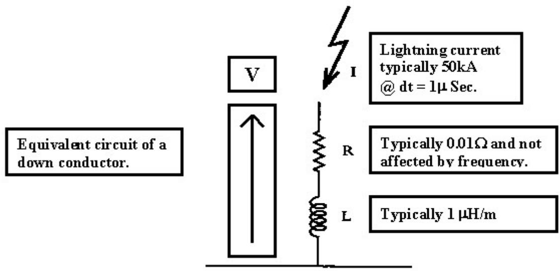
V is the voltage generated over a 10 m long conductor when the resistance is defined as R and the impedance as  $L \frac{di}{dt}$ .
