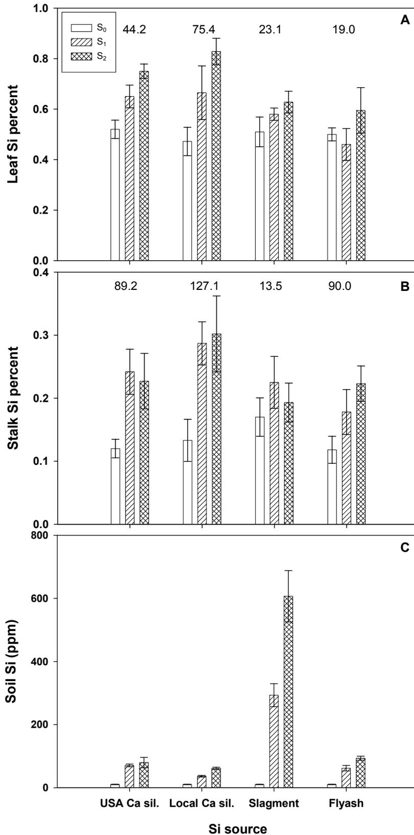
**Figure 1. Mean leaf Si per cent (A), stalk Si per cent (B) and soil Si (C) recorded from samples taken on 19 August, 20 August and 5 March 2002, respectively, from each Si source at control (S<sub>0</sub>), 5000 kg/ha (S<sub>1</sub>) and 10 000 kg/ha (S<sub>2</sub>) treatment levels. Error bars are standard errors. Figures above bars in A and B are the percentage increase in Si% between S<sub>0</sub> and S<sub>2</sub>.**
