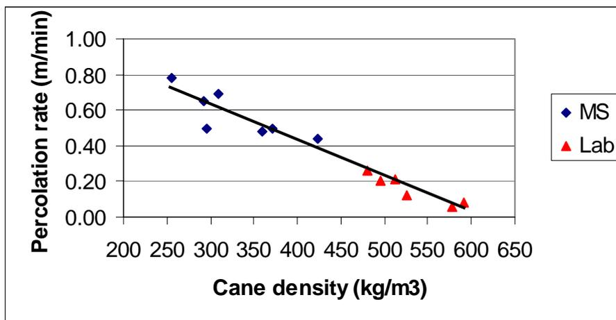
**Figure 3. The relationship between percolation rate and cane density in laboratory and pilot plant diffusion columns.**
