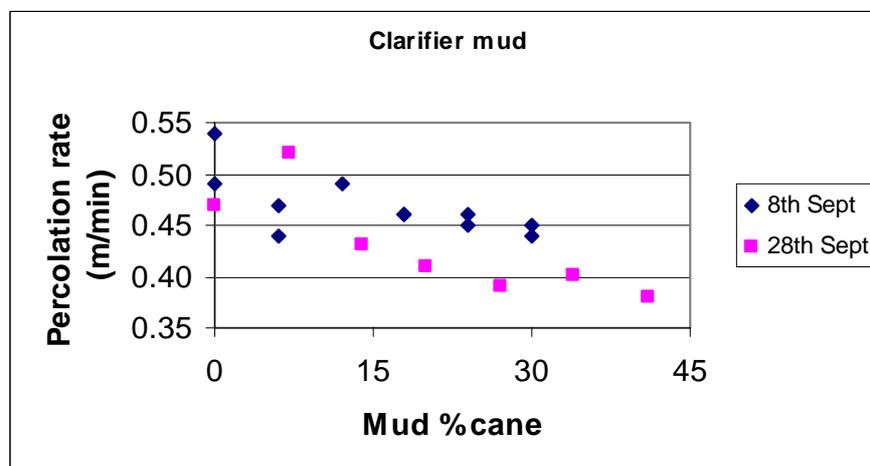
**Figure 5. The effect of clarifier mud on the percolation rate in the pilot column at Maidstone.**
