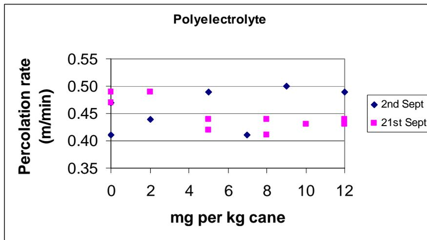
**Figure 4. The effect of flocculant on the percolation rate in the pilot column at Maidstone.**
