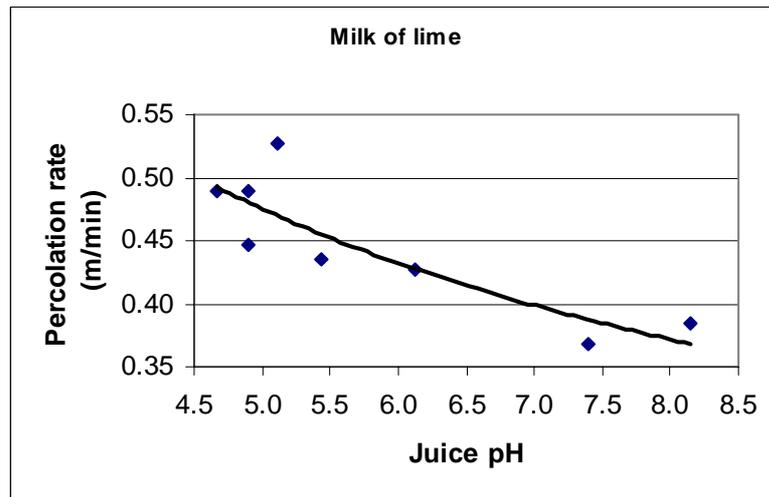
**Figure 7. The effect of pH measured at room temperature on the percolation rate in the pilot column at Maidstone.**
