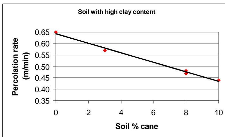
**Figure 6. The effect of a high clay content soil on the percolation rate in the pilot column at Maidstone.**
