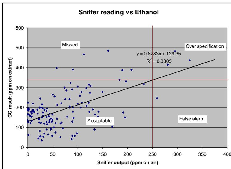
**Figure 6. Comparison of ethanol detector and GC results.**
