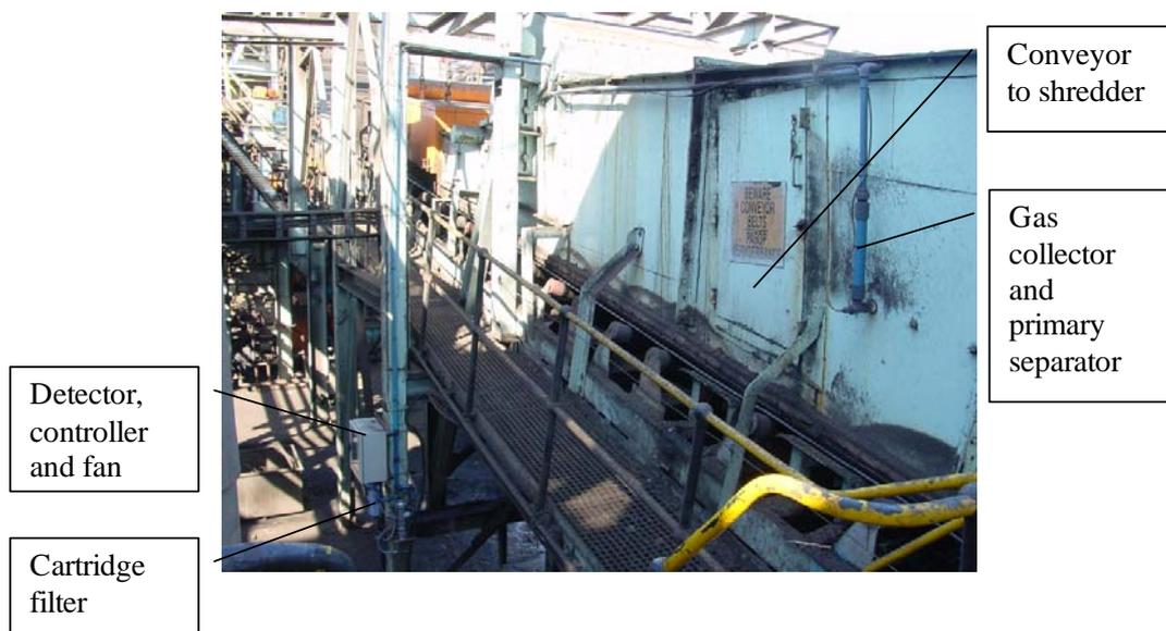
**Figure 2. Ethanol detector mounted just after knives.**
