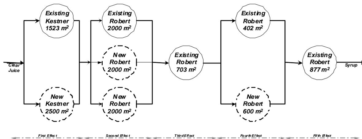
**Figure 8. Evaporator configuration for the final expansion stage (250 TCH).**
