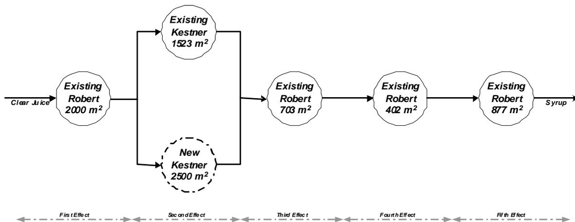
**Figure 7. Evaporator configuration for the intermediate expansion stage (150 TCH).**
