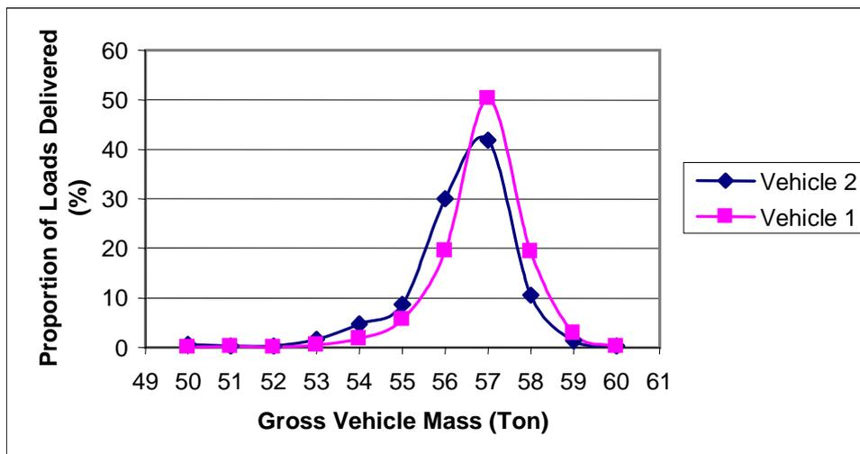
**Figure 7. Gross vehicle mass of all loads delivered by each vehicle.**
