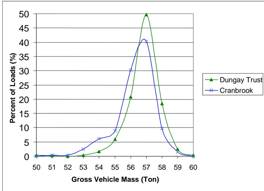
**Figure 5. Gross vehicle mass of loads from individual growers.**
