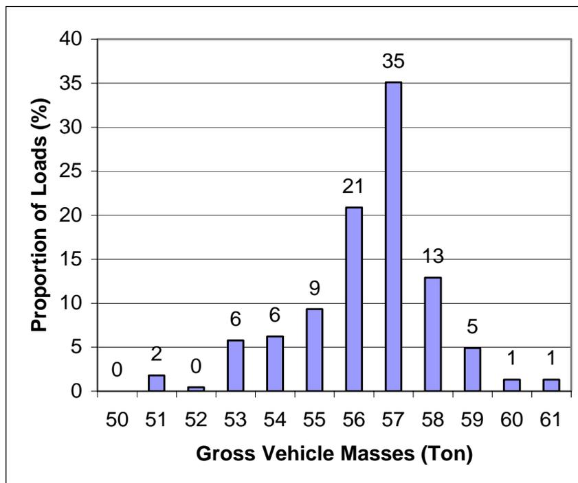
**Figure 9. Gross vehicle masses of loads where Loadtech data was missing.**
