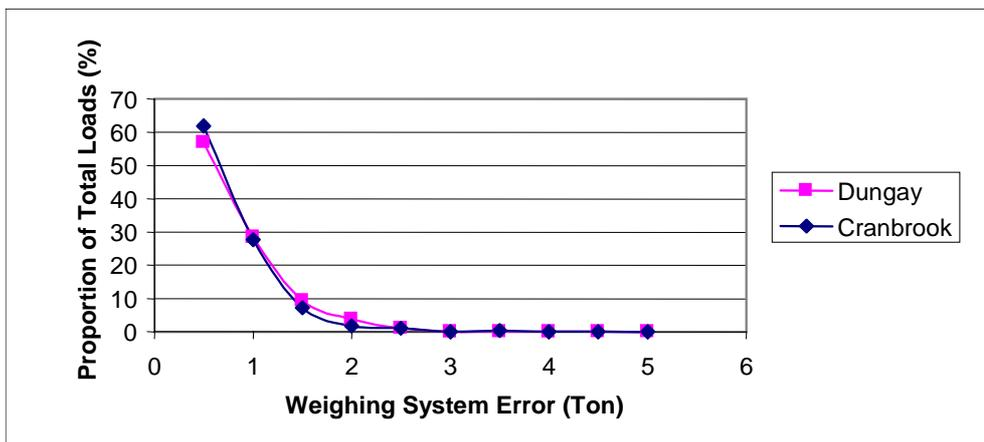
**Figure 6. Weighing system errors at each farm when loading.**
