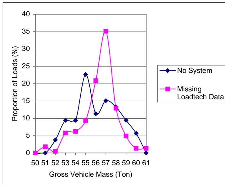
**Figure 11. Gross vehicle mass for loads where no weighing system was used and loadtech data was missing**
