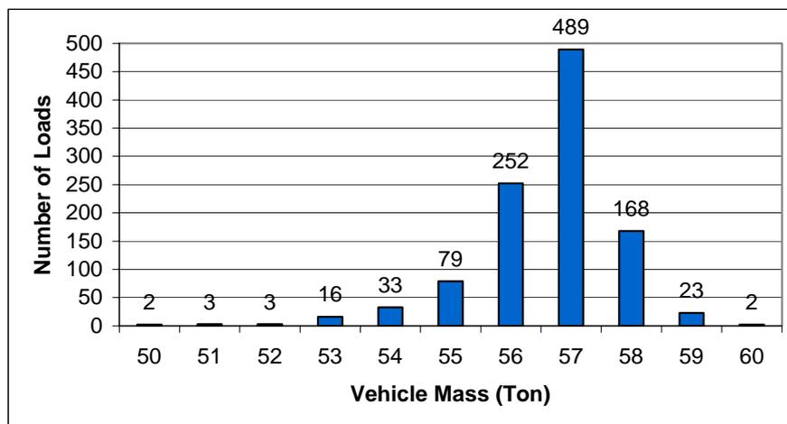
**Figure 2. Gross vehicle mass for all loads during 2005.**
