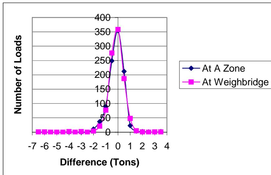
**Figure 4. Difference between Loadtech estimates when at a zone (loading) and at the weighbridge (unloading).**
