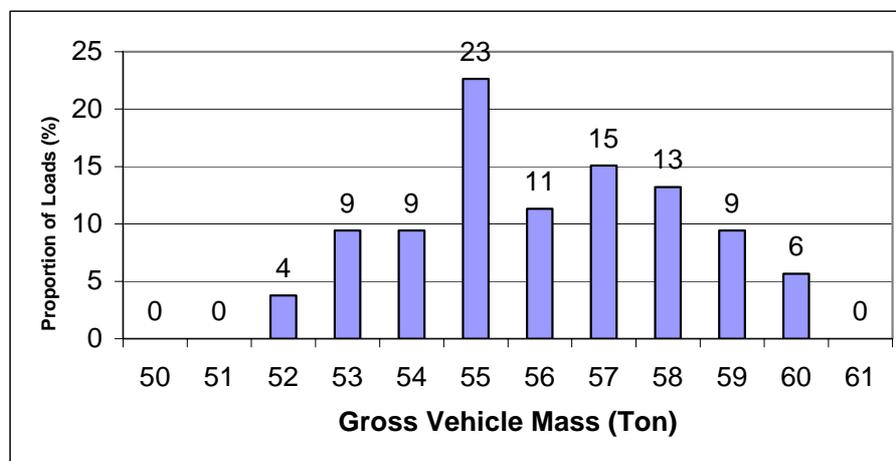
**Figure 10. Gross vehicle masses where no weighing system used**
