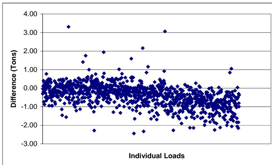
**Figure 3. Difference between Loadtech and weighbridge measurements of gross vehicle mass.**
