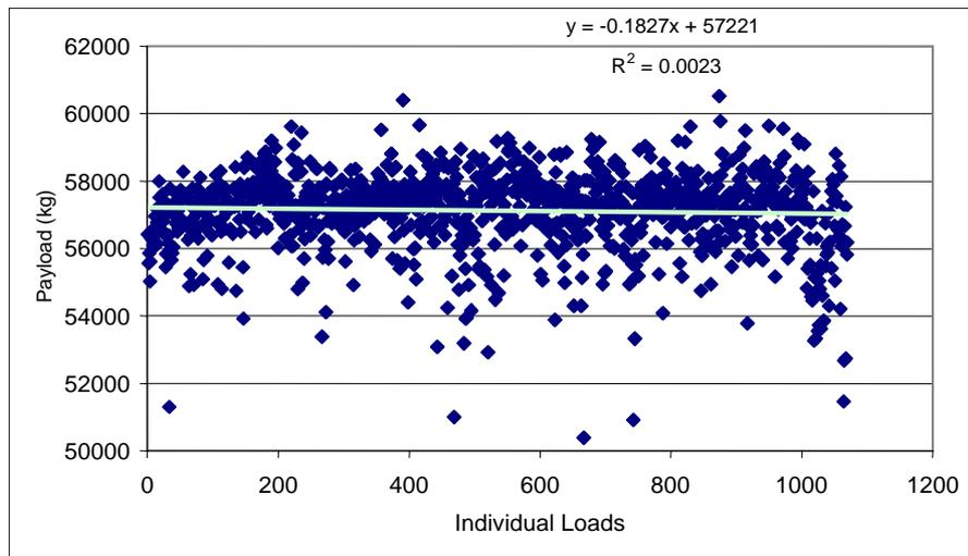
**Figure 1. Gross vehicle mass for loads delivered to Sezela mill during 2005 season (weighbridge).**
