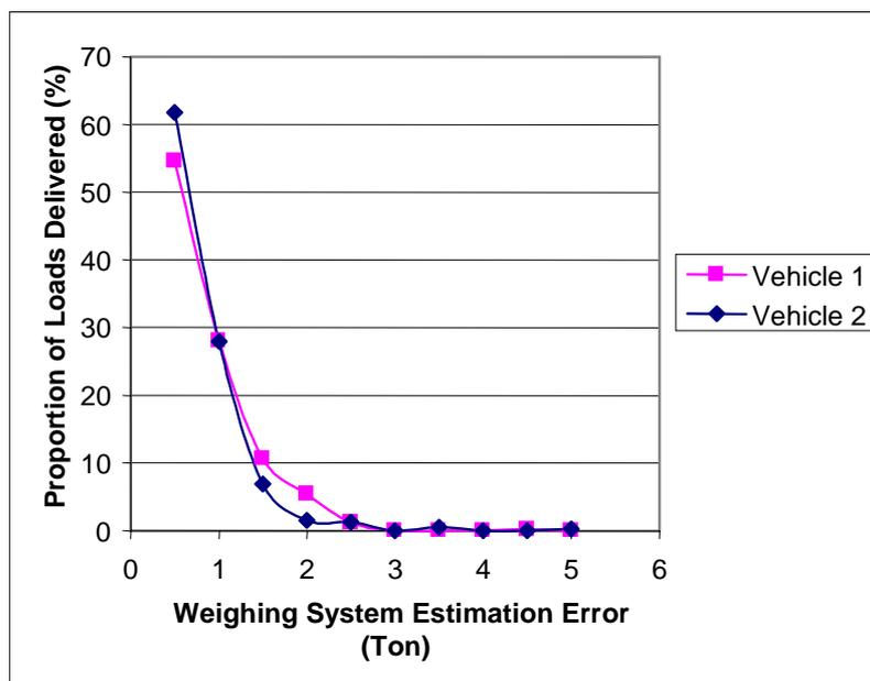
**Figure 8. Weighing system estimation errors on each vehicle when loading.**
