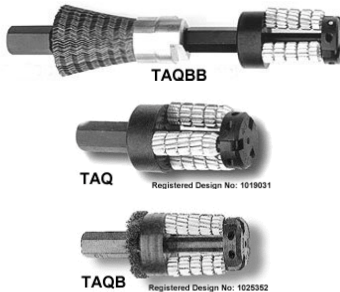
Figure 2. Tool heads: cutters and brush used in the South African sugar industry for cleaning evaporators.
