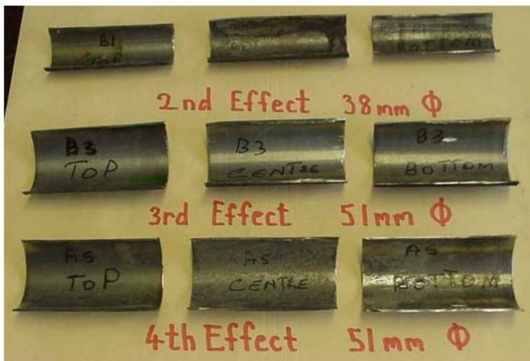
Figure 5. Inside sections of cleaned evaporator tubes.
