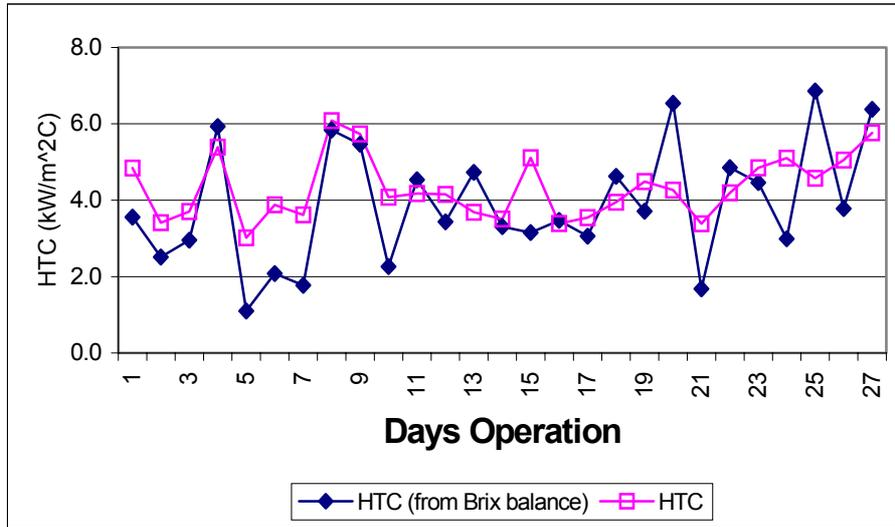
**Figure 3. Heat transfer coefficients for second effect.**
