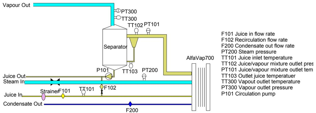
**Figure 1. Configuration of the Alfa Laval test rig.**
