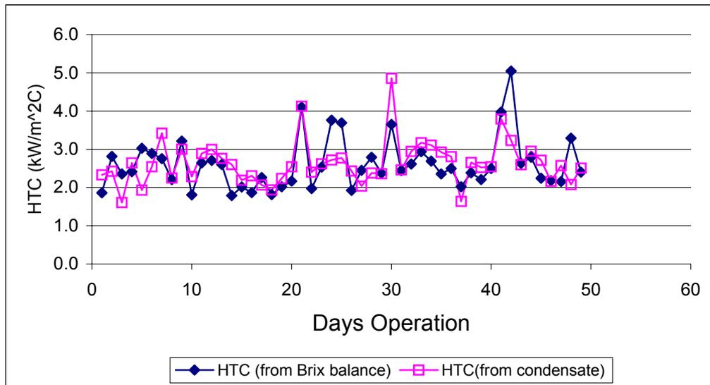
**Figure 2. Heat transfer coefficient for first effect.**
