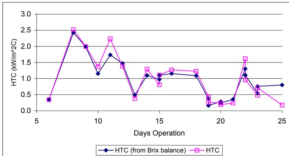
**Figure 4. Heat transfer coefficients for fourth effect.**
