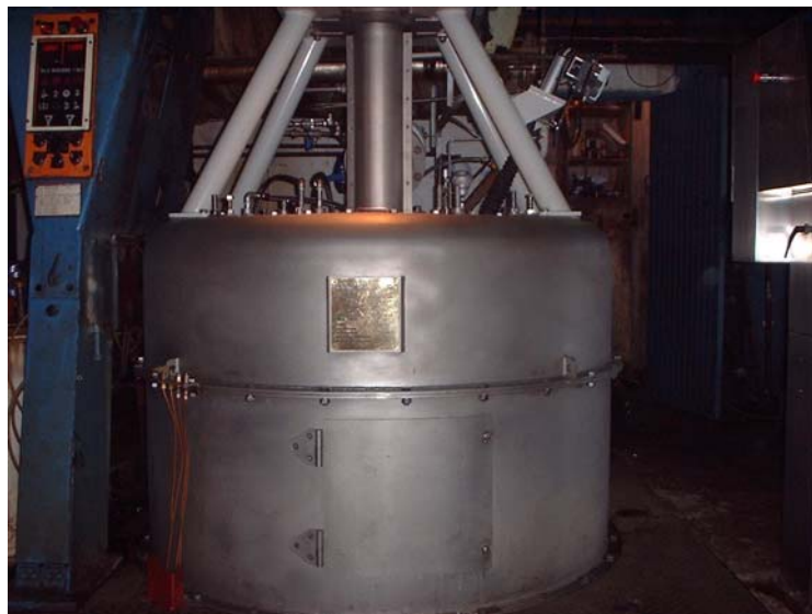
Figure 2. The STG continuous centrifugal installed at the Hulett's refinery in Durban.
