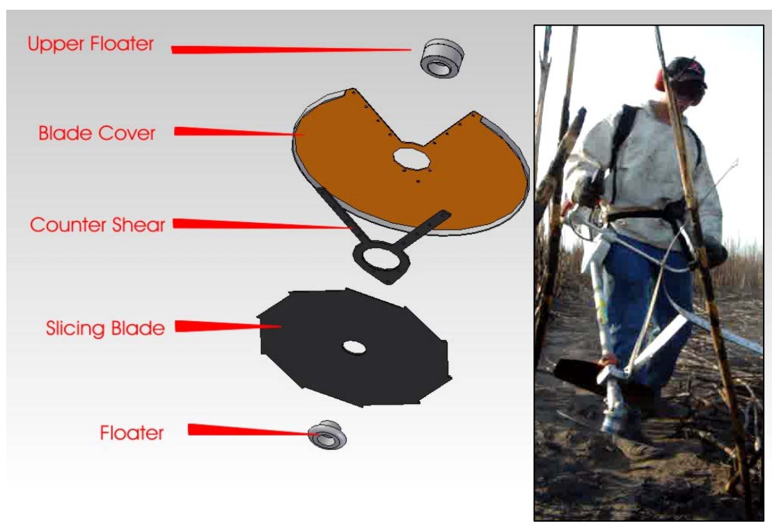
Figure 1. A 22^\circ slicing blade mounted to a brush-cutter, which is used to cut sugarcane.
