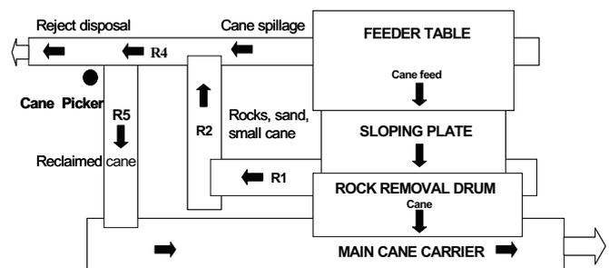
Figure 2. Plan view on R-conveyors.
