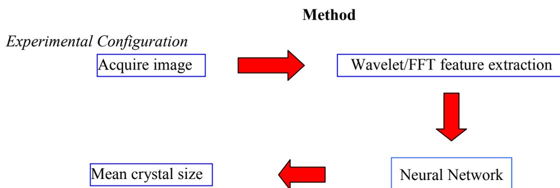
**Figure 1: Procedure used to obtain a measurement of mean crystal size directly from images of the crystal.**
