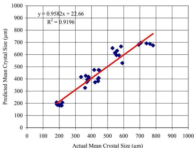
**Figure 9: Performance of the neural network for images obtained from a laboratory crystalloscope immersed in a glycerine solution of sugar crystals.**
