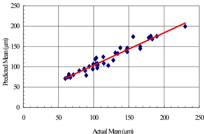
**Figure 8: Performance of the neural network using the Tongaat- Hulett pan images.**
