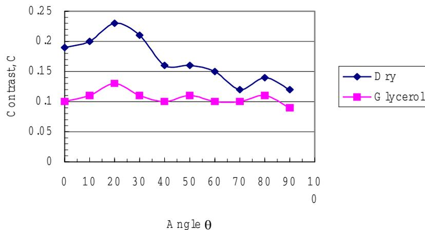
**Figure 5: The change in contrast as a function of polariser angle.**
