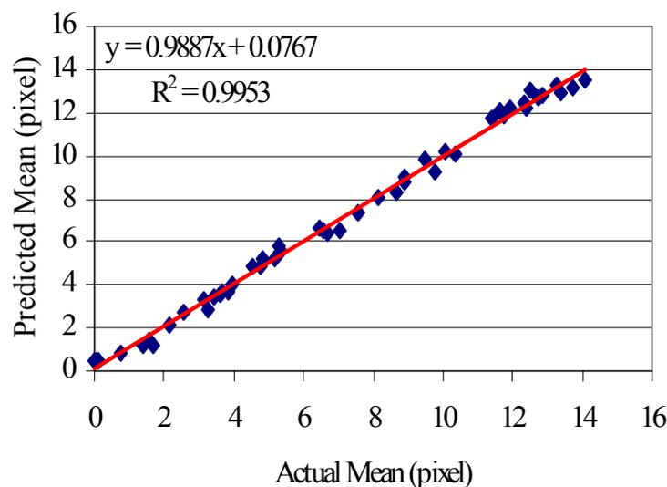
**Figure 7: Performance of the neural network on unseen, noisy artificial images.**
