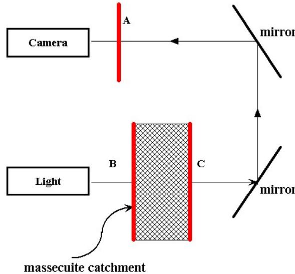
**Figure 4: The crystaloscope light system showing the light path from the source through the masseuite to the camera.**
