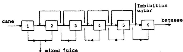
**FIGURE 1** Milling tandem
