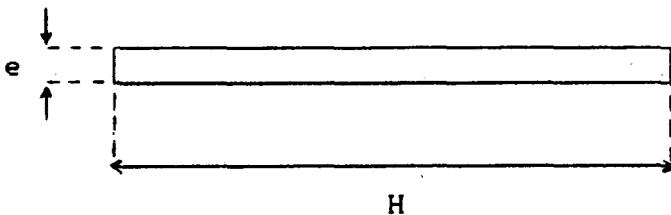
FIGURE 3 Cross-section of a platular channel.
